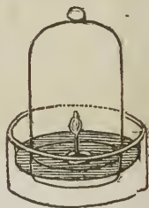
Combustion of a taper under a receiver.
