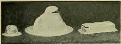
FIG. 178.—How steel tears in drawing.
