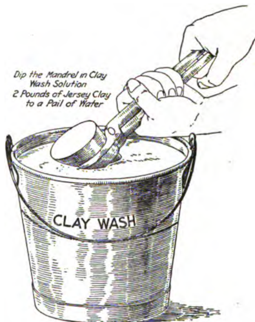
FIG. 2. INSURING A SMOOTH SURFACE WITH CLAY WASH DIP
