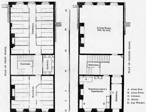
PLANS OF THE MODEL LODGING-HOUSE, No. 76, HATTON GARDEN. TO ACCOMMODATE 57 SINGLE WOMEN.
