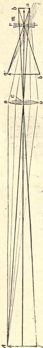
Fig. 83.—Construction of Galileo's telescope.
