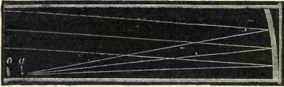
Action of the reflecting telescope with anterior opening.
