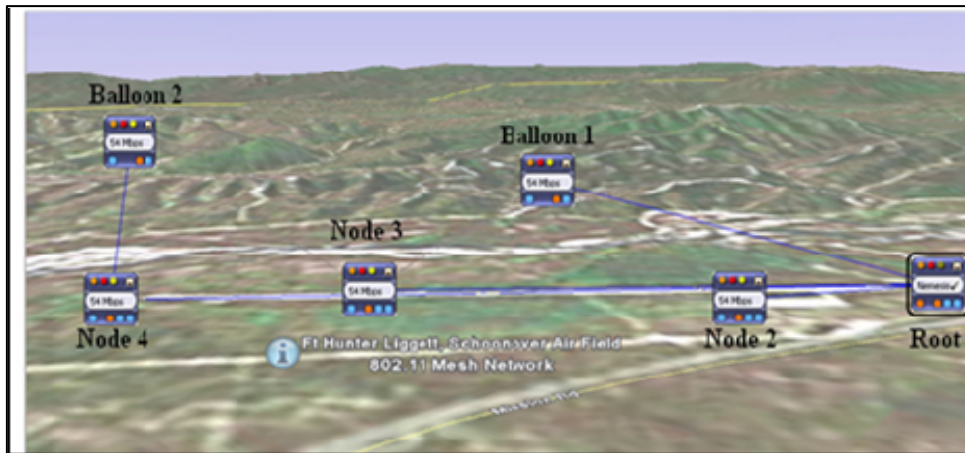
Figure V-2. Mesh Ground AP Layout at Fort Hunter Liggett (from Google Earth MAR 2006).
