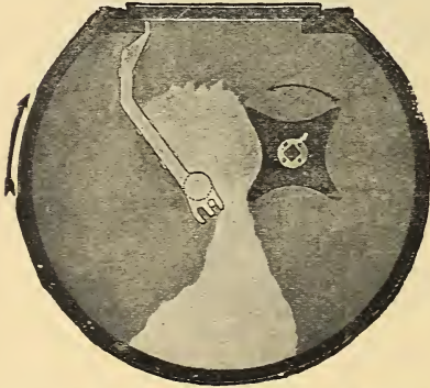
Cross-section view, showing how the butter is worked between two rolls
