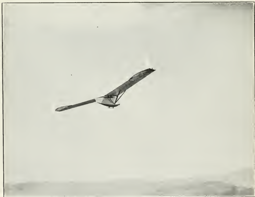
2. THE TAILLESS AIRPLANE "STORCH" AS A SAILING AIRCRAFT
