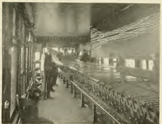
ILLUMINATED TRACK DIAGRAM IN SWITCH TOWER
