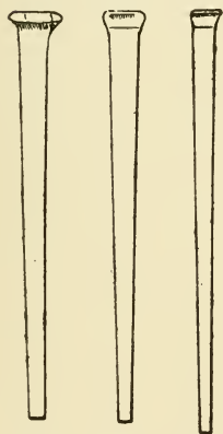
COMMON. CASING. FINISH. Fig. 329.—8d. Cut Nails.
