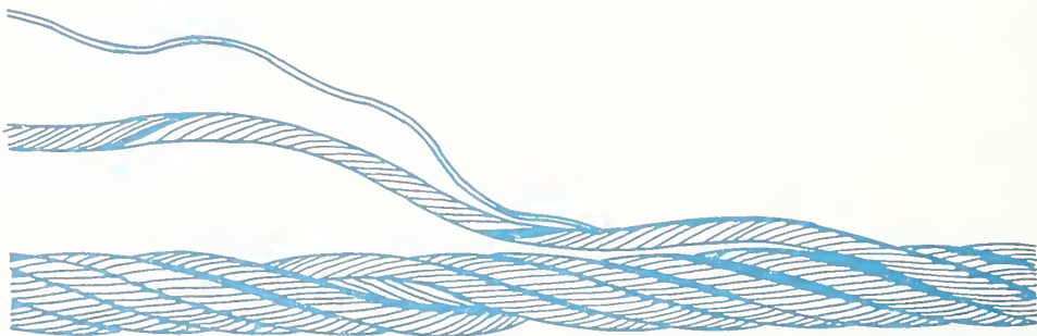
PREFORMED WIRE RETAINS ITS SHAPE EVEN WHEN STRANDS ARE SEPARATED
