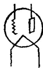
三極真空管 (Three Electrode Tube)
