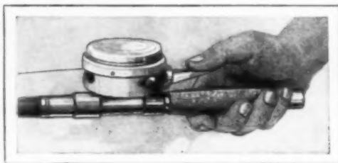
Reel Which Automatically Winds Up the Line After Cast Has Been Made
