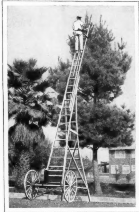
High Folding Ladder for the Tree Trimmer Is Attached to an Auto Trailer
