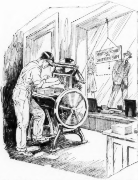
This Motion Sign Is Actuated by the Printing Press and Attracts Considerable Attention.
