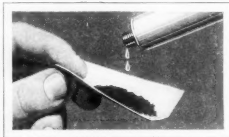
Dropping Testing Liquid on Sample of Soil; It Is Then Drained Off and Compared to Color Chart
