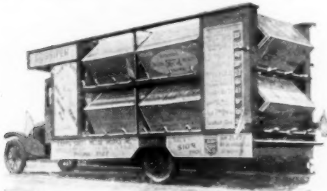
Moving Billboards on Auto Truck; the Posters Revolve as Vehicle Proceeds and Are Lighted at Night
