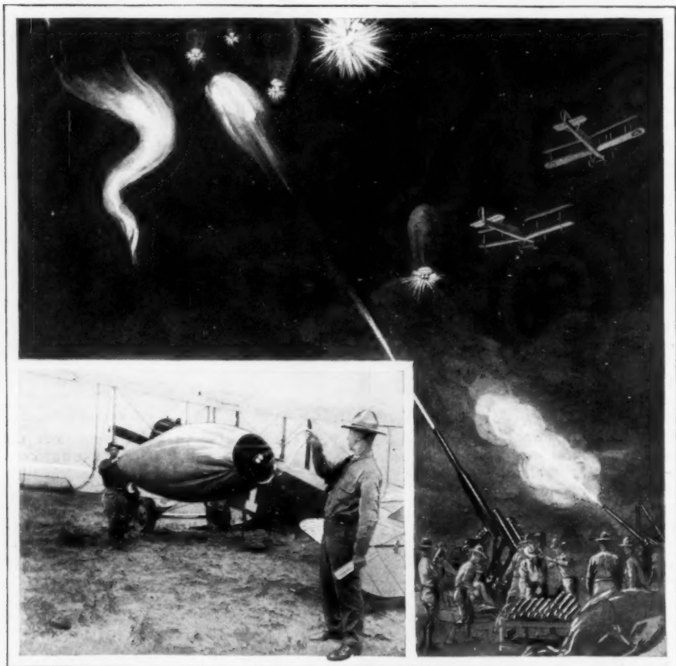
One of the Sleeve-Shaped Targets with the Light in Front, and Drawing Illustrating How Night Gunnery Practice with the Flying Marks Might Appear
