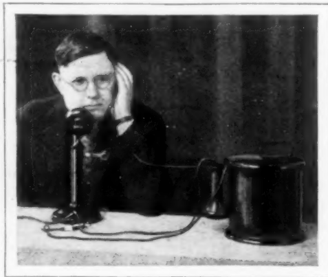
Radio Comes to the Aid of the Deaf in Telephoning; the Amplifying Unit in Use
