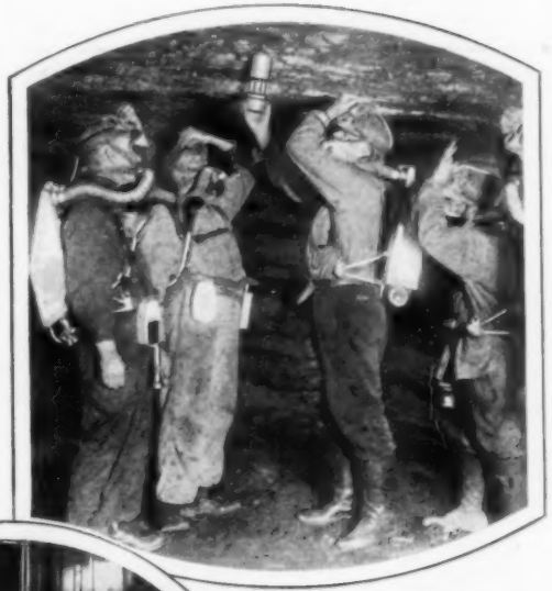
Using a Safety Lamp to Detect Dangerous Gases Clinging to Roof of a Coal Mine, and the Crew, at Left, Studying the Map before Going Underground
