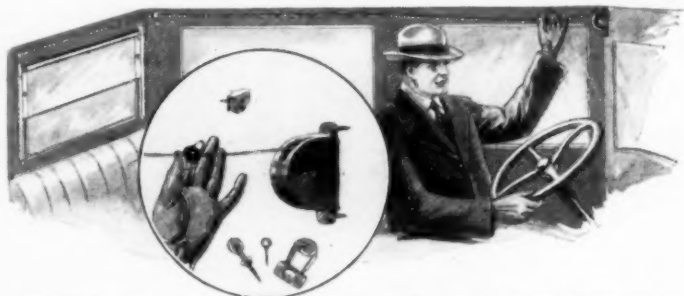
Drawing to Show the Shade Cord in Operation, and a Closer View of the Pulley Attached at Front of Car
