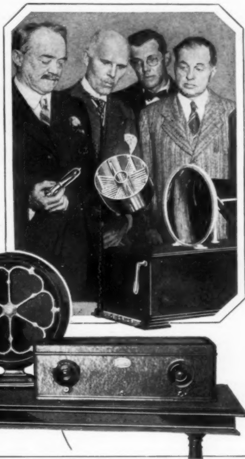
Francis Jenkins with His Scanning Drum, Filled with Quartz Rods as Light Conductors, and, Below, the Receiver, Loud Speaker and Picture Apparatus, Showing the Receiving Lens and Mirror
