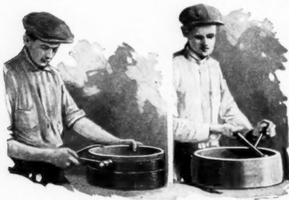
Cast-Iron Rings Used as Forms on Which Auto Brake Bands Can Be Hammered True
