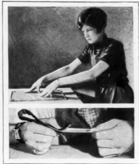
Showing How Pads Keep Glass and Paper from Slipping: They Require No Adhesive
