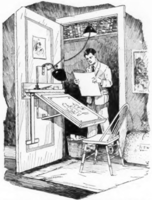
Collapsible Drawing Table Is Attached to a Closet Door in Home or Apartment
