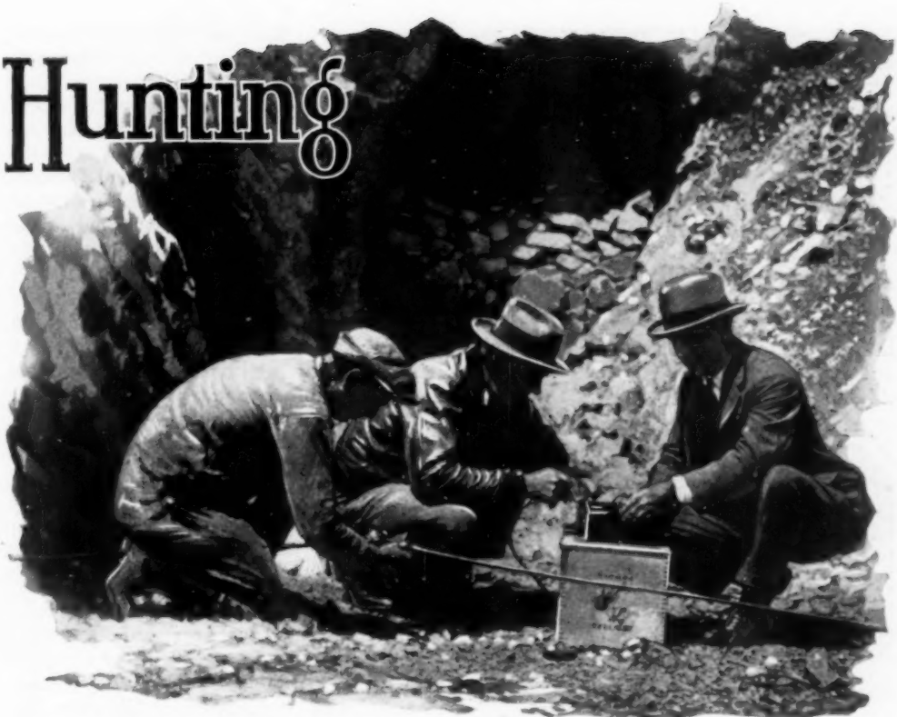
Making an Artificial Earthquake with Explosives, So That the Underground Waves May Be Measured to Indicate the Presence of Ore and Other Shock-Resisting Substances Far Below
