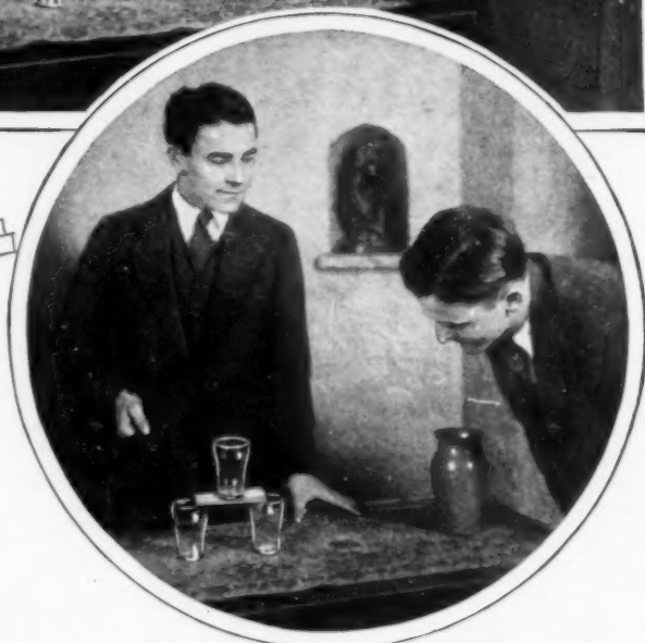
A Sheet of Ordinary Paper Will Support a Water Glass, Provided It Is Properly Folded in Accordion Pleats
