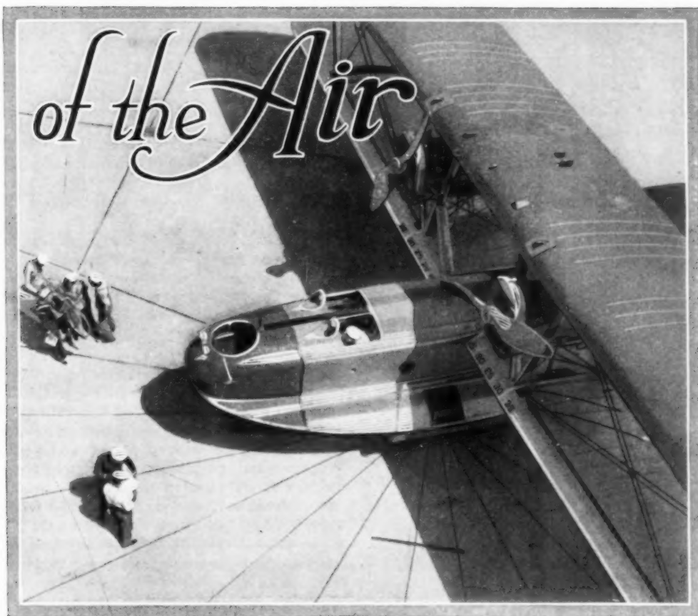
Swinging Ship to Correct the Compass of a Huge Twin-Motored Flying Boat; Note the Compass Points Laid Out in Radiating Lines on the Concrete Base to Guide the Correctors
