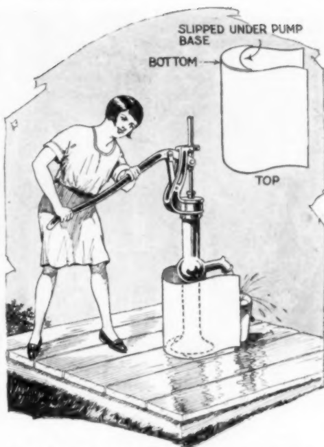
Splash Guard Consisting of a Large Tin Can, Cut Open and Fitted around the Pump Base
