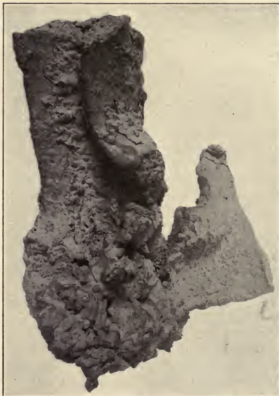
FIGURE 146. FUSED CAST-IRON PULLEY FROM THE BAYONNE FIRE.
