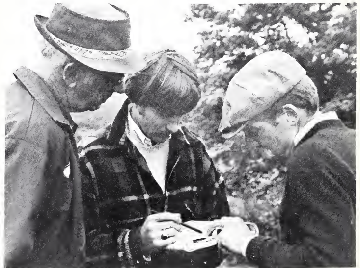
At left, Tim McCormick, OSSP specialist, uses a soil auger to test soil for depth, permeability, stoniness, and other characteristics that could affect sewage treatment.
