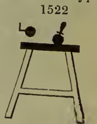
1522 Cowper's inking table and roller.
