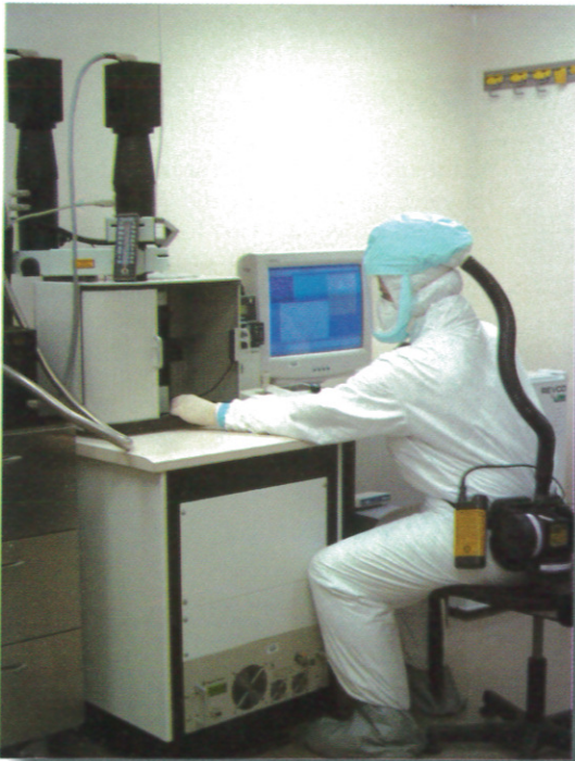
◀ Laboratory technician April Shea takes protective gear through its paces while working with a Raman imaging detector to analyze for the presence of biological agents, circa 2002. (NCP 17413)
