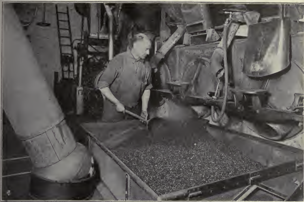
DUMPING THE ROAST IN A COAL ROASTING PLANT
