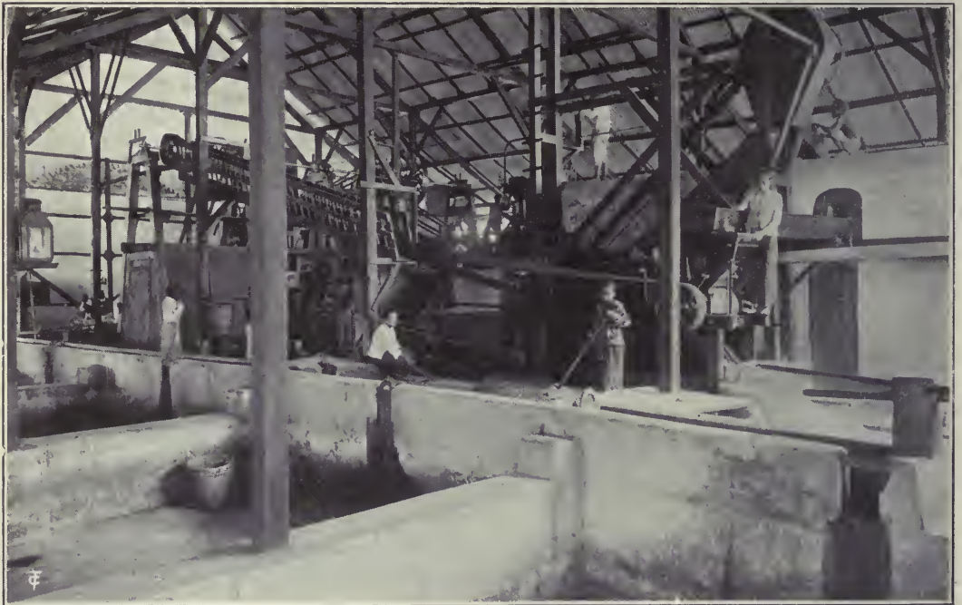
INTERIOR OF A MODERN COFFEE FACTORY IN EAST JAVA Showing pulping machinery and fermentation tanks PREPARING JAVA COFFEE FOR THE MARKET
