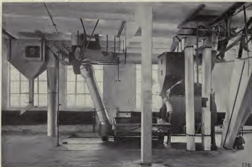
UPPER-STORY VIEW OF A JUBILEE PLANT, SHOWING ROASTER, COOLER, AND STONER EQUIPMENT
