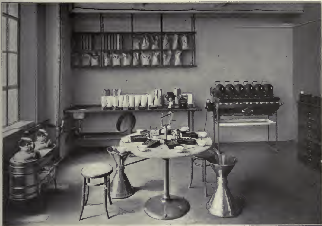
TYPICAL SAMPLE-ROASTING AND CUP-TESTING OUTFIT
