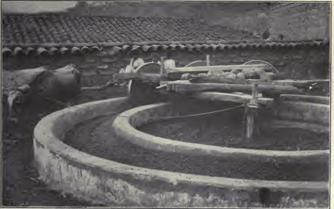
THIS OLD-FASHIONED HULLING MACHINE IS OPERATED BY OX POWER IN VENEZUELA
