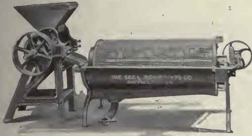
GRANADA UNPULPED COFFEE SEPARATOR Shown in combination with a Guatemala coffee pulper
