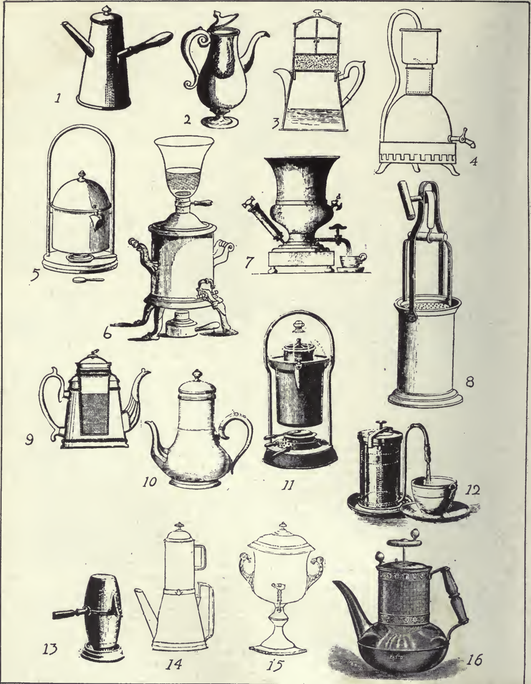
1 — English adaptation of French boiler. 2 — English coffee biggin. 3 — Improved Bumford percolator. 4 — Jones's exterior-tube percolator. 5 — Parker's steam-fountain coffee maker. 6 — Platow's filterer. 7 — Brain's Vacuum, or pneumatic, filter. 8 — Beart's percolator. 9 — American coffee biggin. 10 — cloth-bag drip pot. 11 — Vienna coffee pot. 12 — Le Brun's cafetière. 13 — Reversible Potsdam cafetière. 14, 15 — Gen. Hutchinson's percolator and urn. 16 — Etruscan biggin
