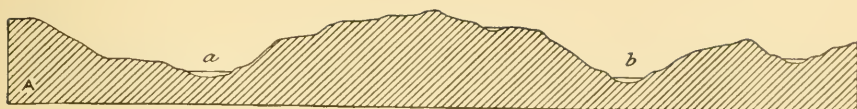
1.—Section showing conditions in early Tertiary times. A, Auriferous slates; a, b, stream beds.
