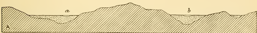
2.—Conditions at close of great gravel-forming period and before volcanic activity began. A, Auriferous slates; a, b, river beds clogged with auriferous gravels.
