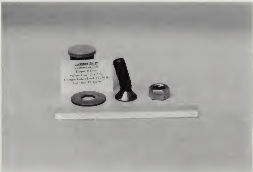
Specimen BS-19, Countersunk Bolt, 0 ft-lbs torque. View of bolt showing severe bending. Note fracture which has initiated between threads.
