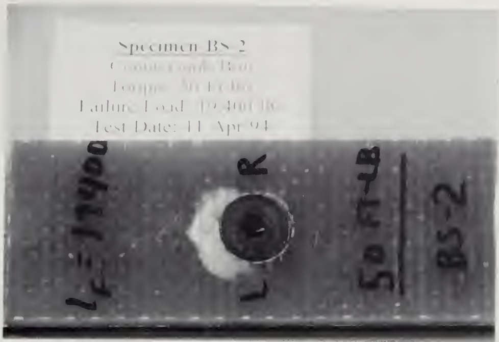
Specimen BS-2, Countersunk Bolt, 50 ft-lbs torque. View of outer GRP surface/bolt head, showing delamination and bolt bending.
