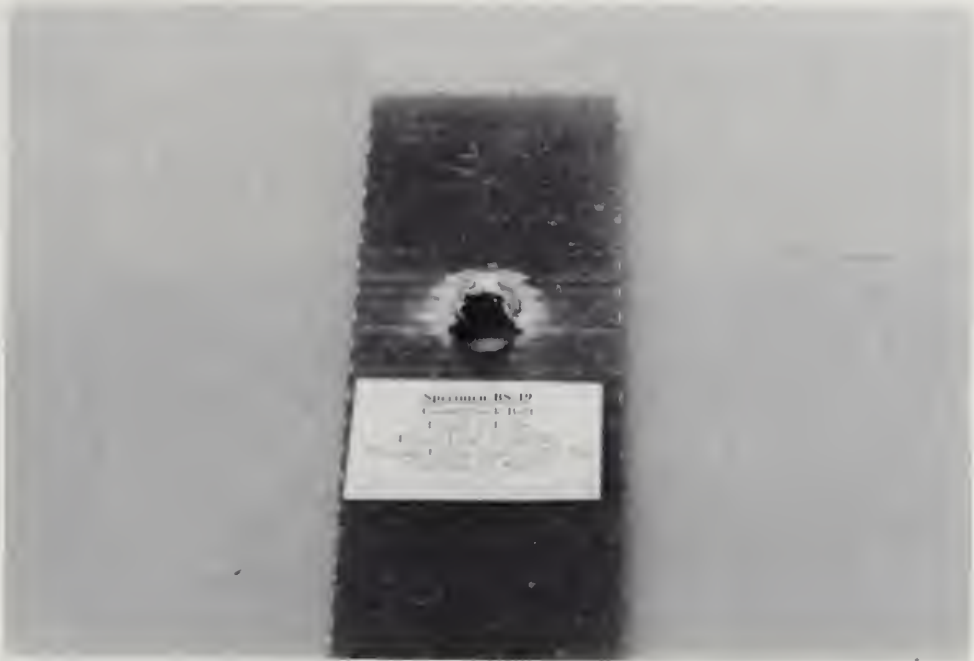
Specimen BS-19, Countersunk Bolt, 0 ft-lbs torque. View of inner GRP surface showing delamination, brooming, and hole deformation.
