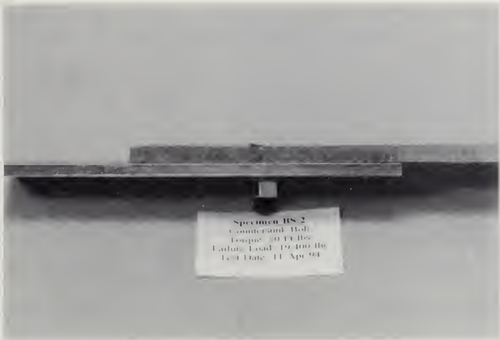
Specimen BS-2, Countersunk Bolt, 50 ft-lbs torque. Edge view of joint showing bolt bending and surface brooming.
