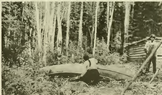
Pitch being applied to seams.
