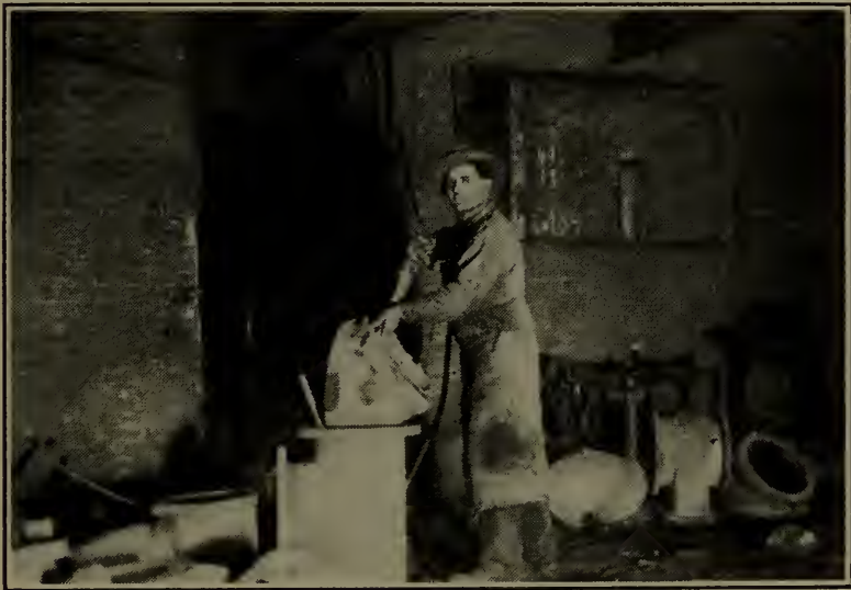
Fig. 122—In the foundry of McNab & Harlin, Paterson, N. J. small chipping hammers are employed for all kinds of casting trimming.
