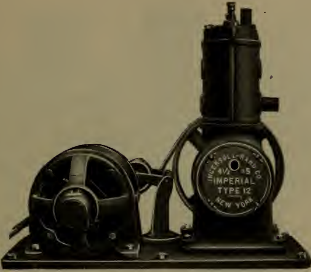
Fig. 7 — A vertical compressor 'short-belt' motor-driven. The compressor is arranged for cylinder cooling by circulating water.
