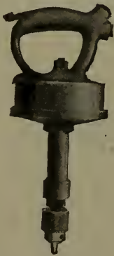
Fig. 64—Pneumatic drill for drilling tell-tale holes in stay bolts.
