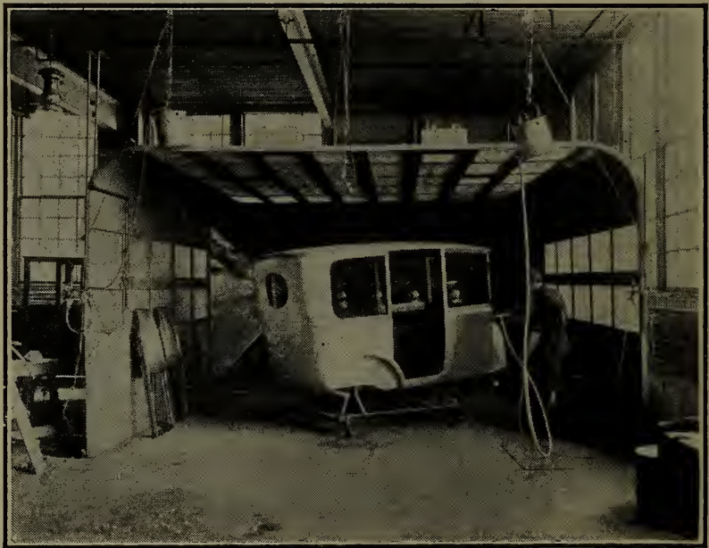
Fig. 265—Paint spraying in the body department of an automobile manufacturing plant.
