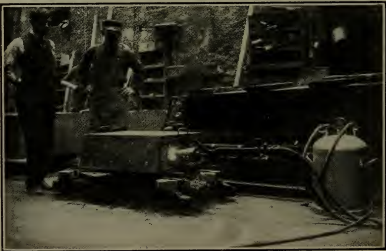
Fig. 124—Baking ornamental molds with a Hauck Burner. The molds are placed in a sheet-iron box lined with asbestos or fire clay.
