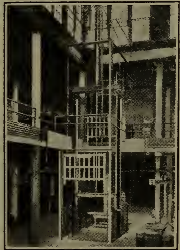
Fig. 57—Vertical Cylinder Hoist applied to elevator lift of considerable height.
