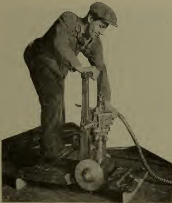
Fig. 160—Pneumatic drill rigged as a portable saw for cutting belt slots, repairing floors, etc.
