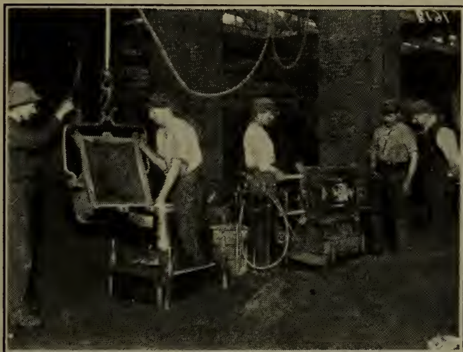
Fig. 110—Jolt ramming machine at work on separator pedestals.
