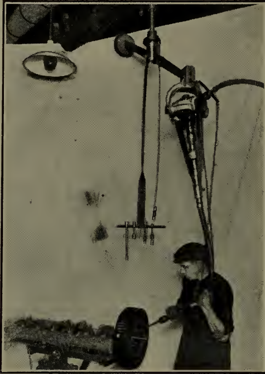
Fig. 151—Utilizing a pneumatic drill for assembling motor fly-wheel to crank shaft flange.
