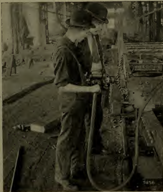
Fig. 194—Pneumatic drill at work reaming holes in car frames in the plant of the J. G. Brill Co., Philadelphia.
