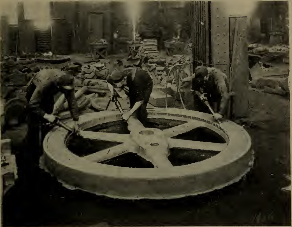
Fig. 121—Chipping Hammers at work on a large fly-wheel. The use of pneumatic chipping hammers for this class of work has enabled the foundryman to make a considerable saving in the cost of trimming and finishing castings.
