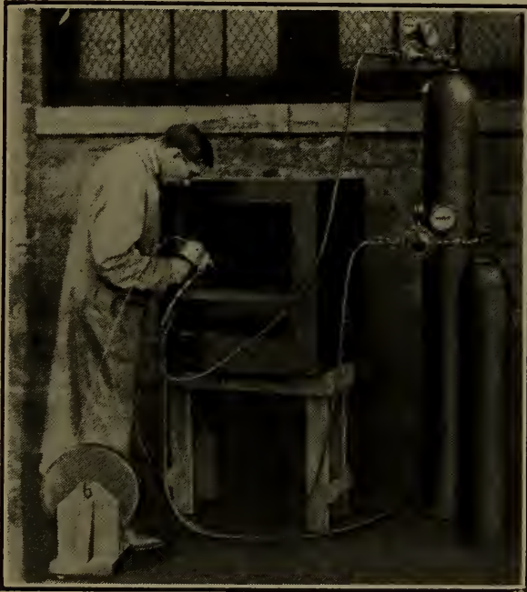
Fig. 275—Metal coating stove oven linings.
