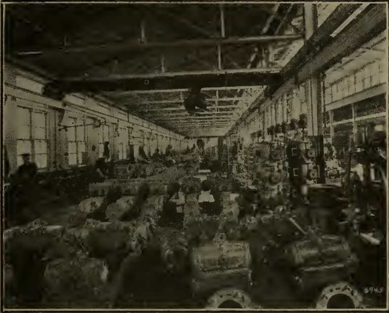
Fig. 159—Assembly Department of a large pump works. Swinging wall arms have been provided for suspending pneumatic stud seating tools and other pneumatic devices.
