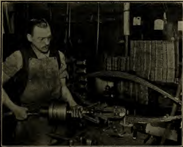
Fig. 155—A special pneumatic device for clipping off bolt ends.
