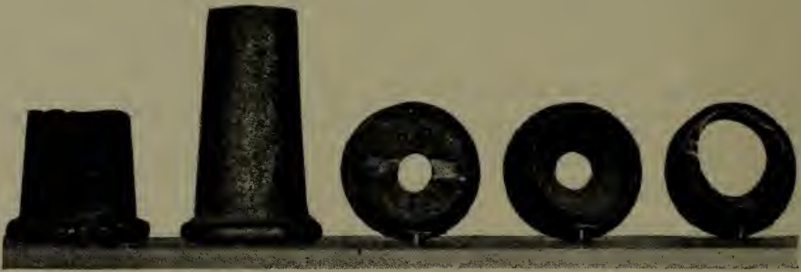
Fig. 128—Effect of wear on Sand Blast Nozzles.
