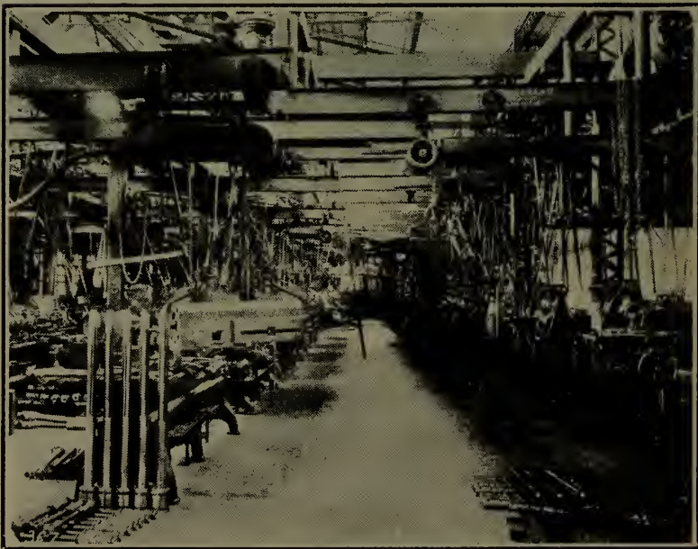
Fig. 241—Horizontal cylinder hoists serving machine tools.
