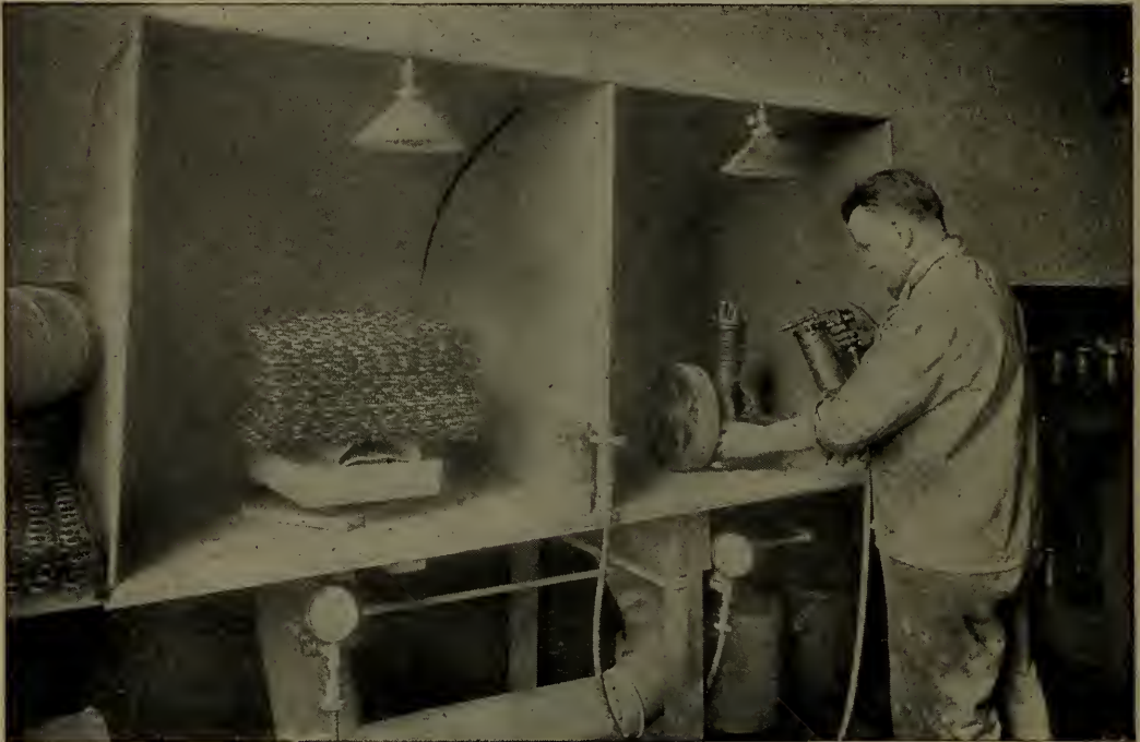
Fig. 273—Painting small engines with air brush.
