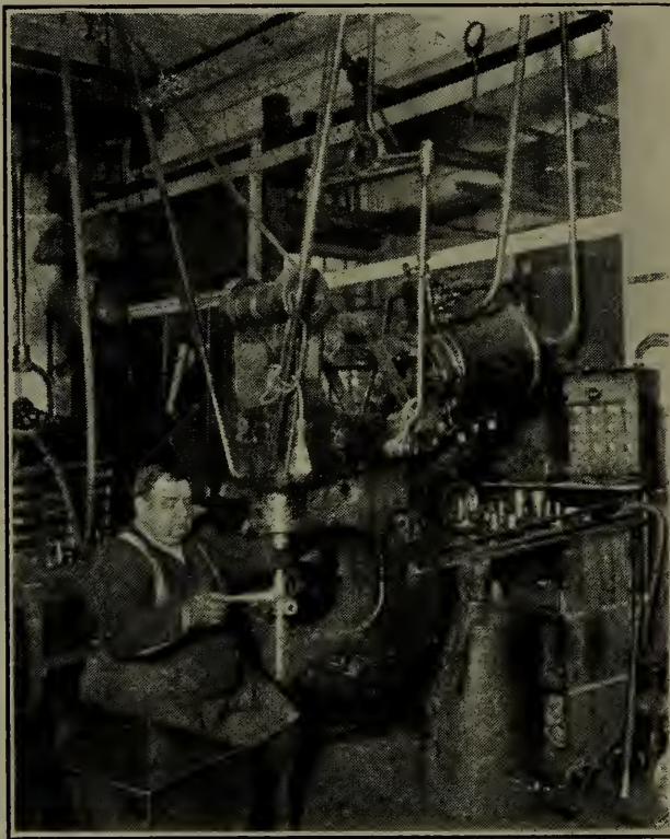
Fig. 215—Hanna Pneumatic Yoke Riveter used on automobile work in the H. H. Franklin Mfg. Co's. Plant, Syracuse, N. Y.
