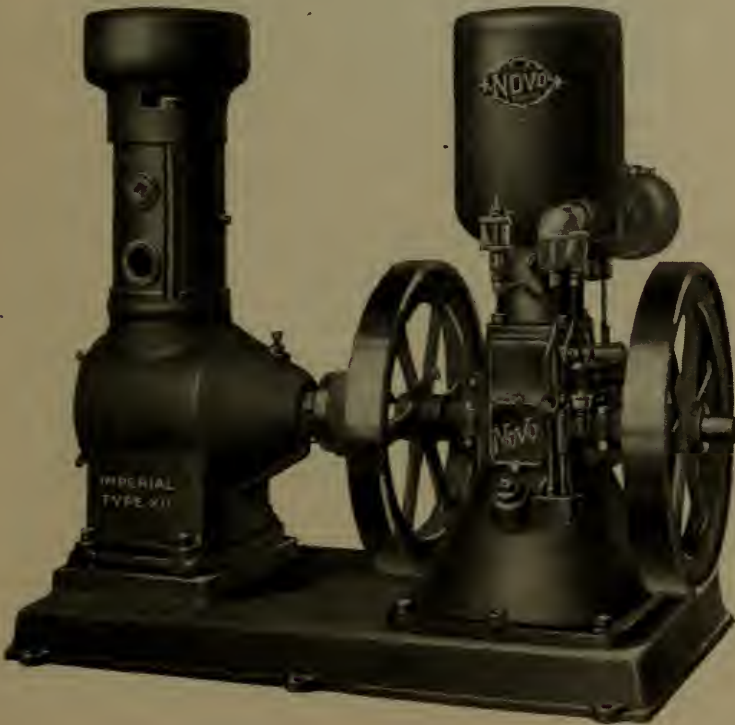
Fig. 8—A vertical air compressor direct-connected by flexible coupling to a vertical gasoline engine,
