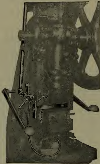
Fig. 254—Automatic pneumatic ejecting device attached to punch press.
