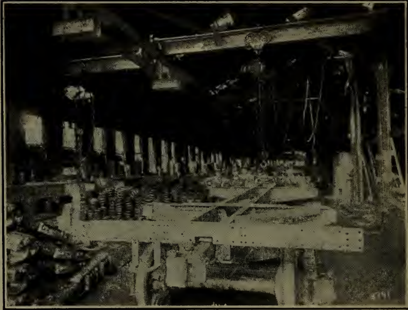
Fig. 246—Pneumatic hoists used in conjunction with traveling cranes in the plant of the American Car & Foundry Co., Jeffersonville, Ind.
