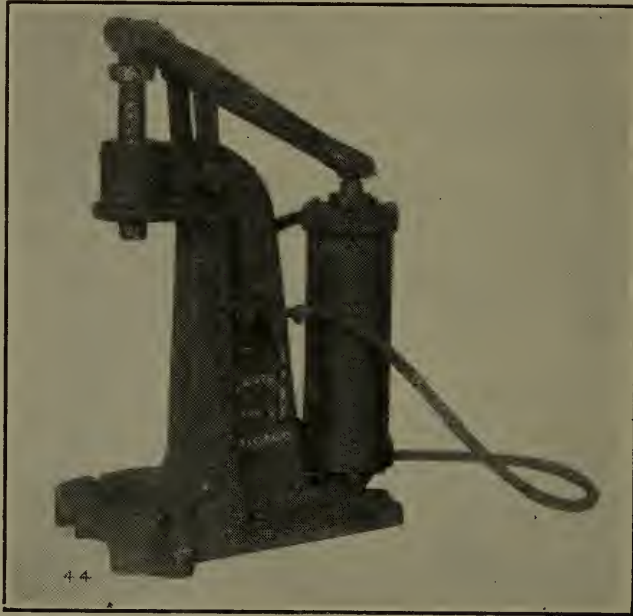
Fig. 176—Air operated arbor press.
