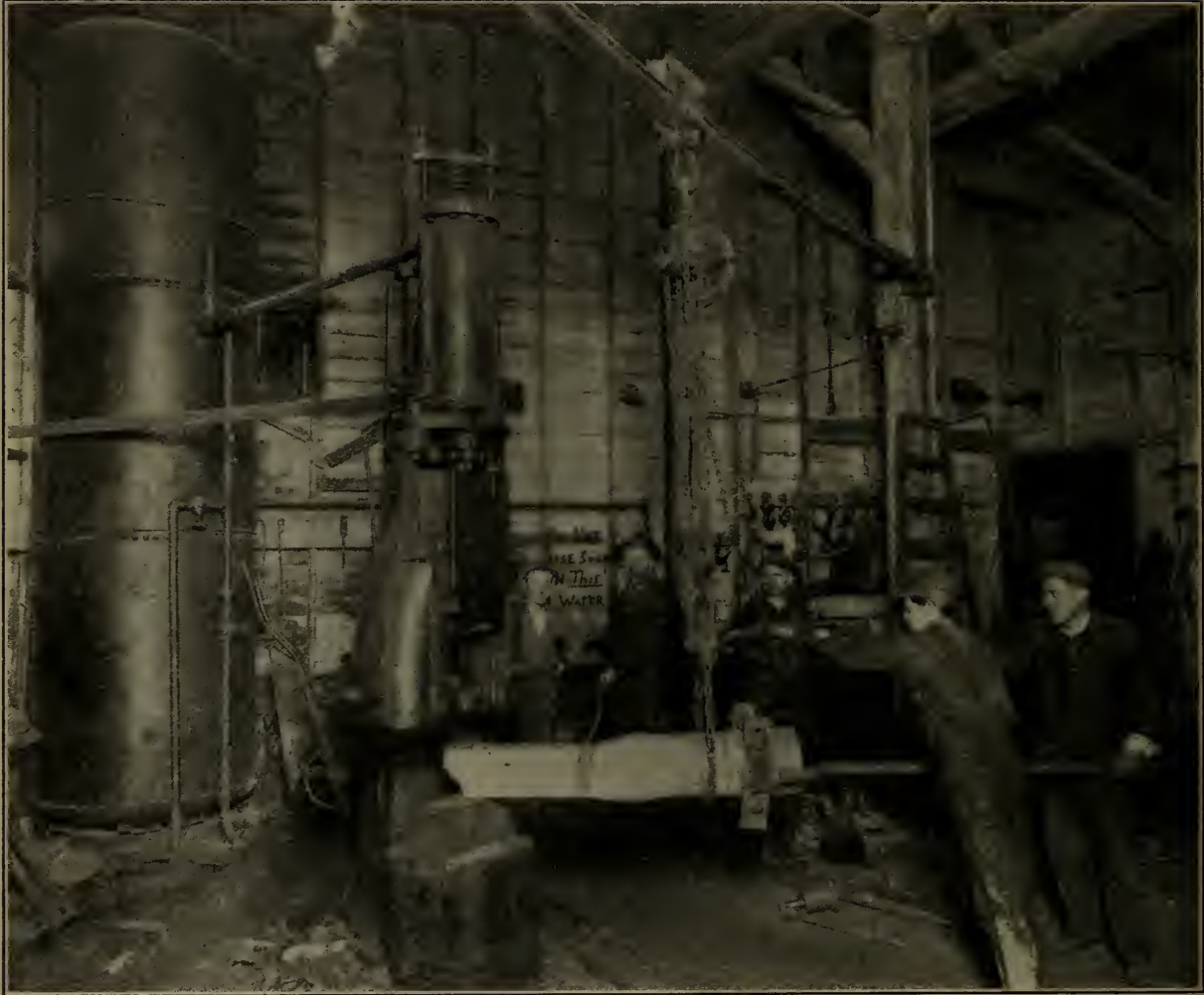
Fig. 178—Steam Forging Hammer converted to pneumatic operation.
