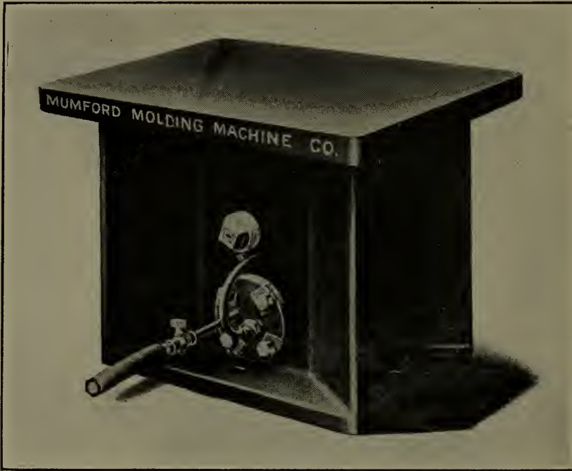
Fig. 109—Jarring machine designed specially for core work.
