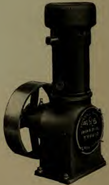
Fig. 6—A vertical compressor arranged for long-belt driving. This particular compressor is equipped with a reservoir water head for cooling the air cylinder. It is a single-stage machine.
