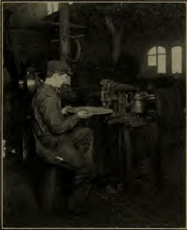
Fig. 190—A portable pneumatic punch in the Meadow Shops of the Pennsylvania Railroad.
