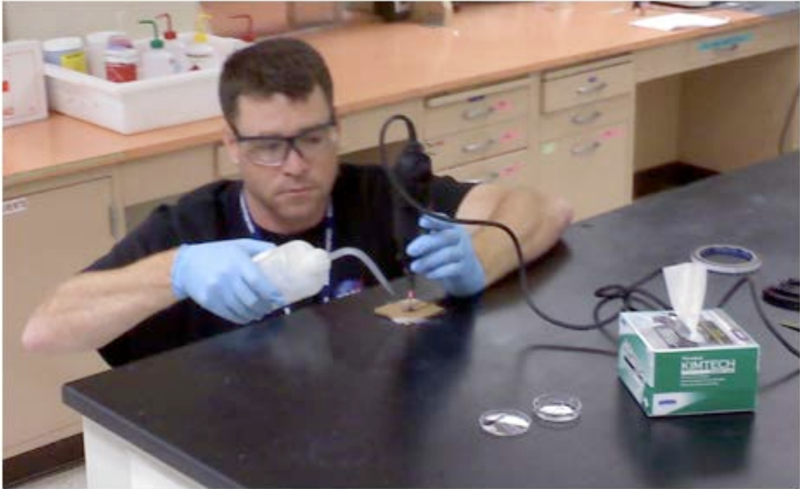
Figure 78. Allow the weight of the Dremel to rest on the silicon. Apply a steady stream of water to the silicon while drilling.
