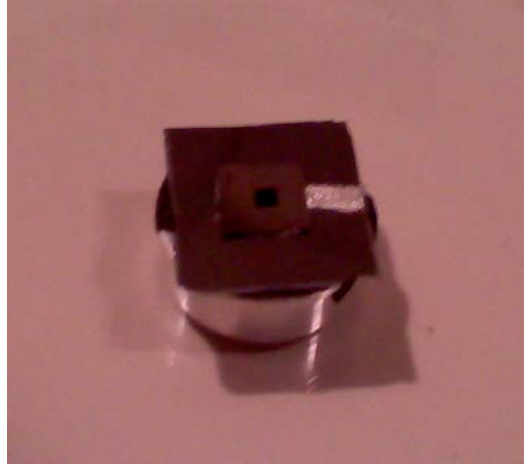
Figure 47. Thin film of silver epoxy applied to the Experiment 5 sample to allow conduction of the charge from the retaining clip to the CPA.
