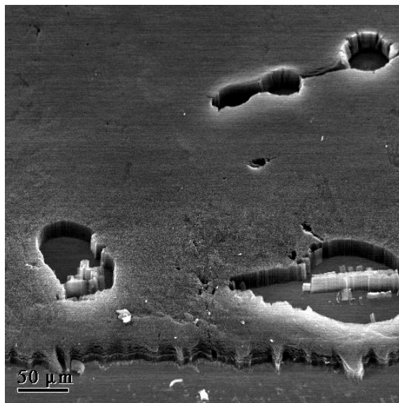
Figure 56. Image showing damage to the Experiment 5 array. These areas most likely had CNTs taller than the rest of the array. Picture is at 250x magnification.
