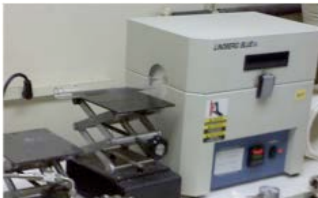
Figure 71. CVD furnace shown with quartz tube inside.
