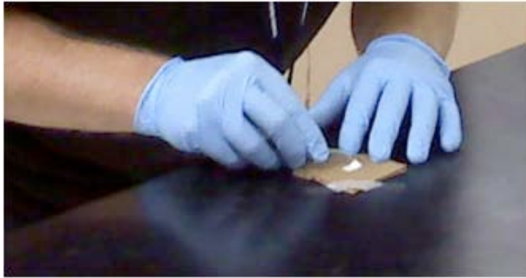
Figure 77. Secure the cardboard to the working surface with tape and apply a strip of double-sided carbon tape to the center of the cardboard.
