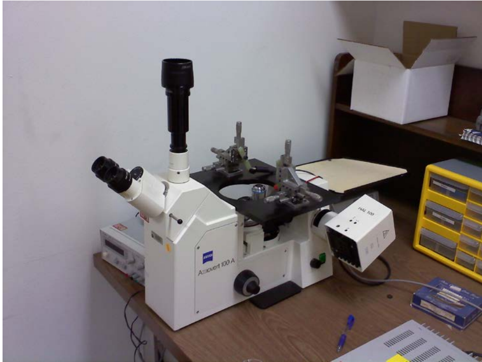
Figure 23. Tabletop microscope used for penetrating the nitride layer.
