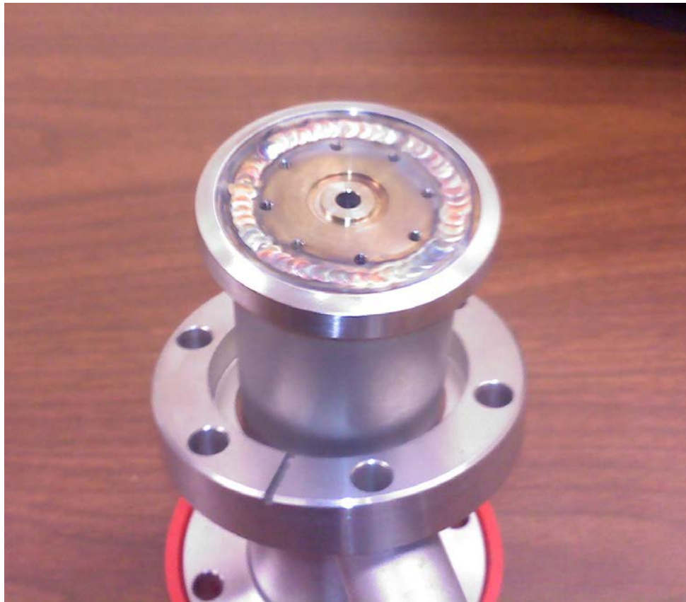
Figure 13. Test base welded into the reducing tee.
