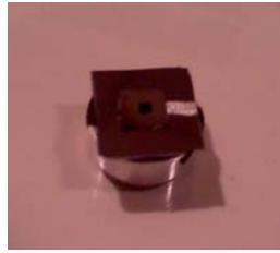
Figure 75. Sample affixed to an SEM mount.
