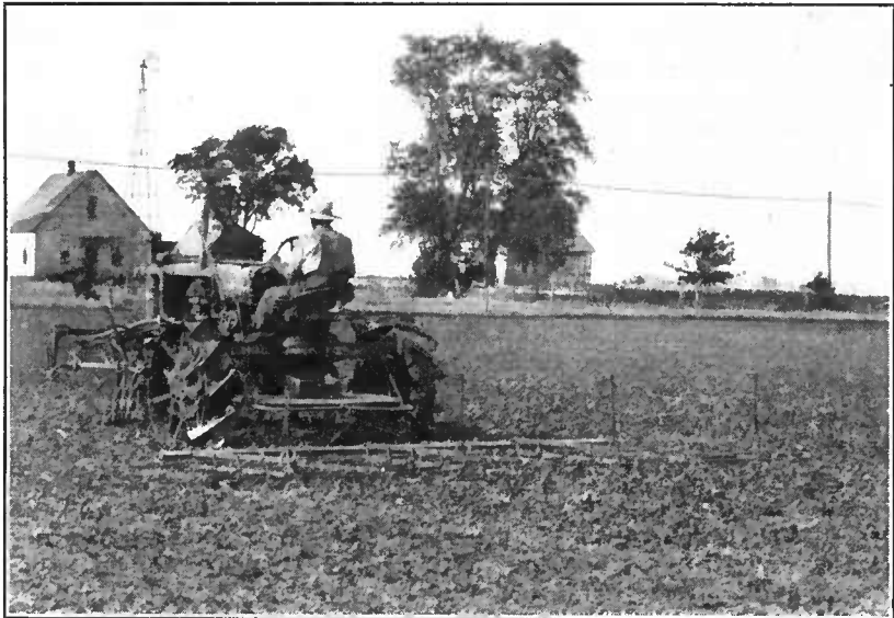
FIGURE 6.—The spike-tooth harrow, with teeth slanting backward slightly, is used extensively in cultivating soybeans.
