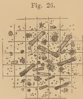
Fig. 26. Microscopic Appearance of Light Carbonate of Magnesia.
