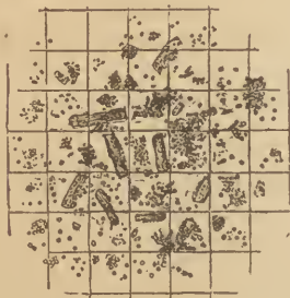
Microscopic Appearance of Common Calcined Magnesia.
