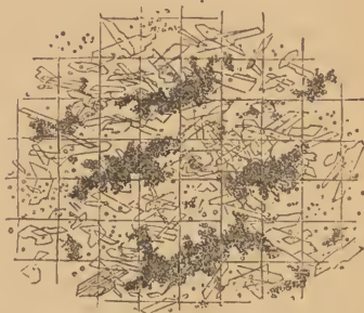
Microscopic appearance of commercial (i. e. impure) precipitated sulphur, showing the crystals of sulphate of lime (selenite).
