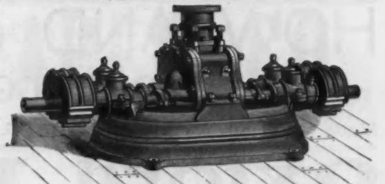
ROTARY FIRE AND SUPPLY PUMP.
