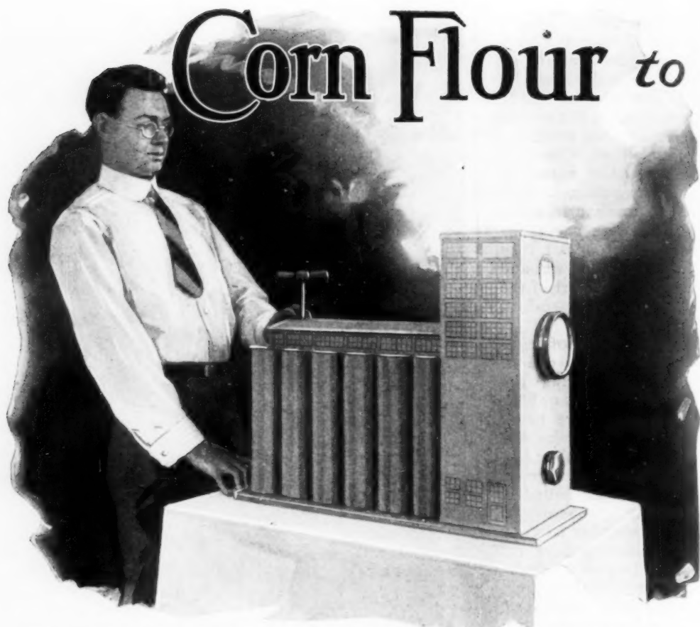
Miniature Grain Elevator Used to Demonstrate Dust Explosions; Such Blasts Have Wrecked Gigantic Concrete Storage Bins and Done Enormous Damage Before Their Cause Was Learned
