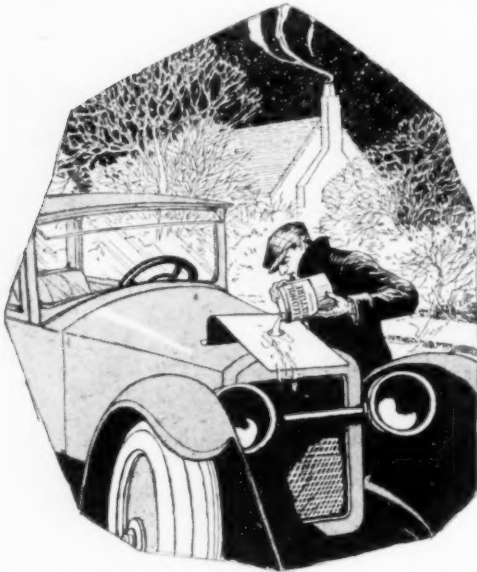
Sheet-Metal Shield over Radiator Prevents Spilling Alcohol Solution on Lacquered Finish
