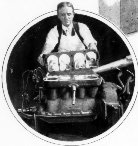
Sheet-Metal Box Used to Mix the Corn Flour and Air to Form an Explosive Product, and the Auto Engine, with Head Removed, Showing, at Right, the Pipe through Which the Mixture Is Sucked
