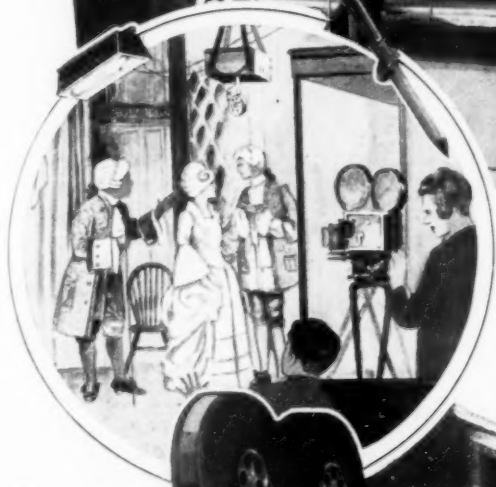
Making Movietone Film for the News Reels with a Portable Outfit Carried in a Motor Truck; from the Microphone the Voice Signals Pass to the Radio Amplifiers Mounted in the Truck, and the Amplified Current Then Returns to the Movie Camera to Operate the Light Which Shines on the Sound Track at the Edge of the Film; the Insert Shows a Studio Scene, with the Camera Operated inside a Glass Cabinet, in Order That the Microphone May Not Pick Up the Clicking of Its Mechanism; Keeping Out Unwanted Sounds Is the Hardest Job in the Making of a "Talkie"
