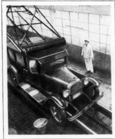
Motor-Driven Brush to Wash Auto Top Does Job Automatically as Car Passes through Laundry
