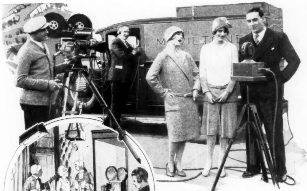
Making Movietone Film for the News Reels with a Portable Outfit Carried in a Motor Truck; from the Microphone the Voice Signals Pass to the Radio Amplifiers Mounted in the Truck, and the Amplified Current Then Returns to the Movie Camera to Operate the Light Which Shines on the Sound Track at the Edge of the Film; the Insert Shows a Studio Scene, with the Camera Operated inside a Glass Cabinet, in Order That the Microphone May Not Pick Up the Clicking of Its Mechanism; Keeping Out Unwanted Sounds Is the Hardest Job in the Making of a "Talkie"
