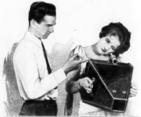
Inventor Demonstrating His New Aerial Camera, Which Is Portable and Uses Standard-Size Plates
