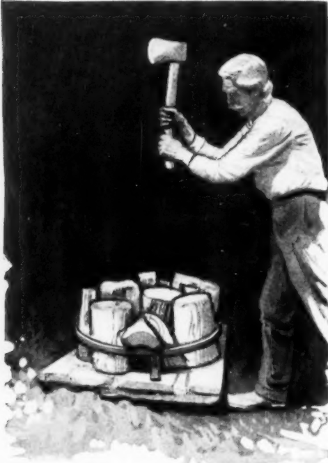
Setting a Number of Pieces of Wood on Edge in a Barrel Hoop Facilitates Chopping
