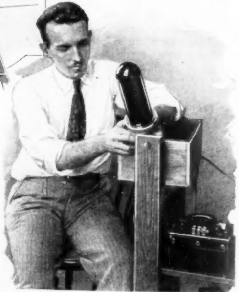
A Movable Ceiling, Adjustable from Six to Fifteen Feet, and a Big Photo-Electric Cell, to Measure the Amount of Light, Are Features of the New Sunlight Test Building
