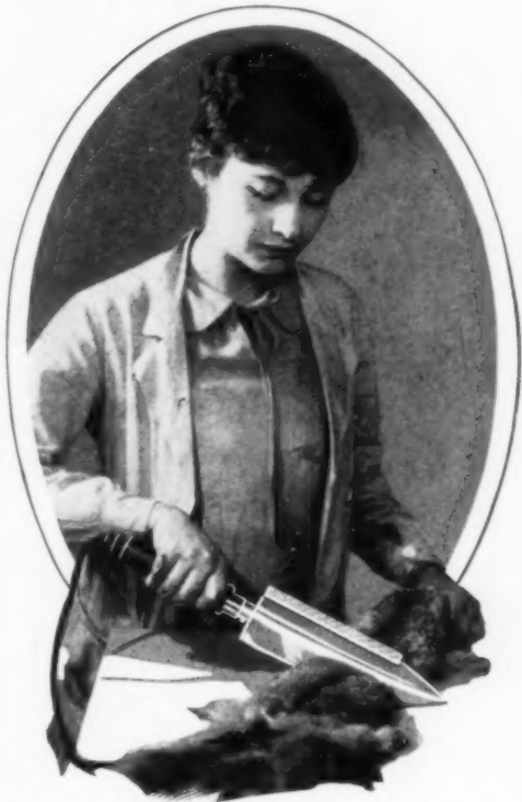
Renovating Fur with the Combination Electric Iron and Comb; Heat Kills Moth Larvæ
