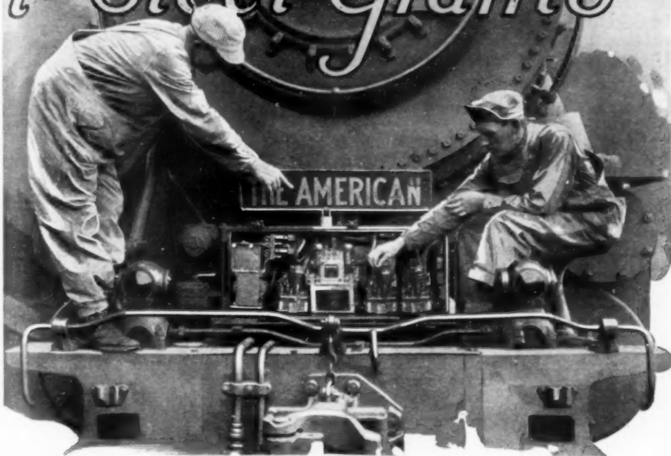
The Little Box That Runs the Train if the Engineer Should Fail; Radio Tubes and Apparatus Play an Important Part in the Automatic Train Control, Which Checks Human Errors
