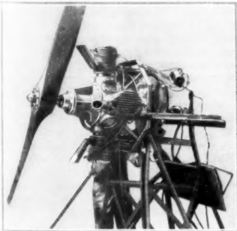
Two-Cycle Valveless Airplane Engine with a Minimum of Moving Parts
