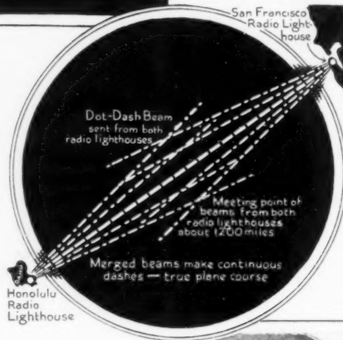
Diagram of the Radio-Beacon System, Which Sends Code Signals That Blend in a Central Path into a Continuous Chain of Dots, and, Above, Arrangement of the Visual Signal Lights Which Convert the Beacon Signals into Green and Red Lights on the Plane's Instrument Board
