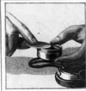
Left, a Simple Water-Level Indicator; When the Lamp Is Pushed Down to Make Contact with the Screw Head Below, It Will Light If the Electrolyte Is High Enough to Touch the Lead
