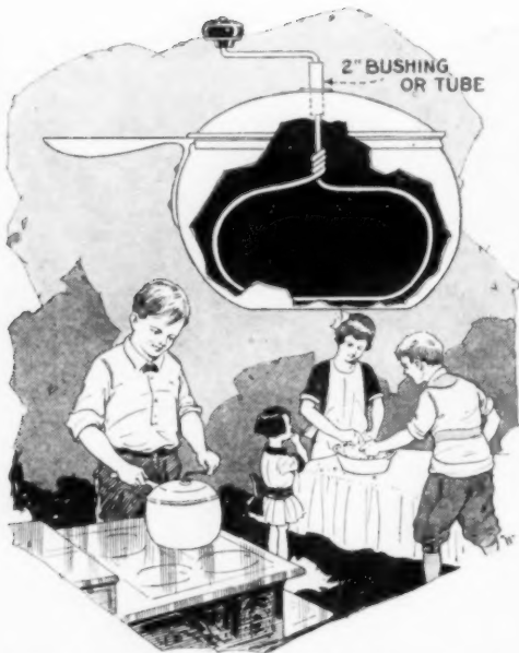
Improved Corn Popper Can Be Made from an Old Cooking Pan and a Piece of Wire
