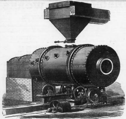
For Roasting, Desulphurizing and Chloridizing Ores. ALSO MANUFACTURERS OF
