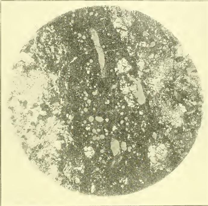
FIG. 11.—Cross section of a vein of one of the Mocs meteorites. The vein mass appears as a broad black band through the center. It is in part intermixed with the adjoining groundmass and in part has well defined walls. The gray spots are spheres and lumps of nickel-iron illuminated by reflected light. The branching of some of these into clefts, one of which is still open, is of interest. \times 20 . After Tschermak. 1
