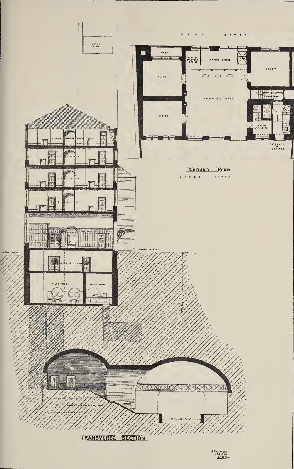
MERSEY TUNNEL RAILWAY STATIONS: SECTION OF JAMES STREET STATION.
