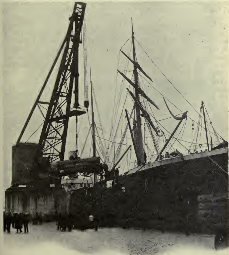
LONDON AND NORTH WESTERN LOCOMOTIVE "EMPRESS" BEING HOISTED ABOARD VESSEL FOR AMERICA
