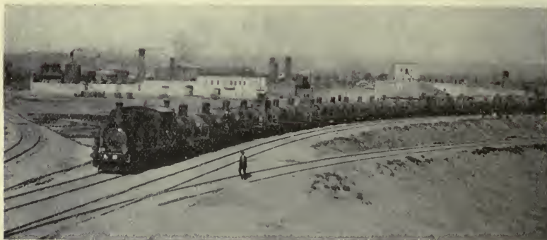
"FAIRLIE" TYPE LOCOMOTIVE HAULING TRAIN OF LOADED OIL TANKS, BLACK TOWN, BAKU (Trans-Caucasian Railway)
