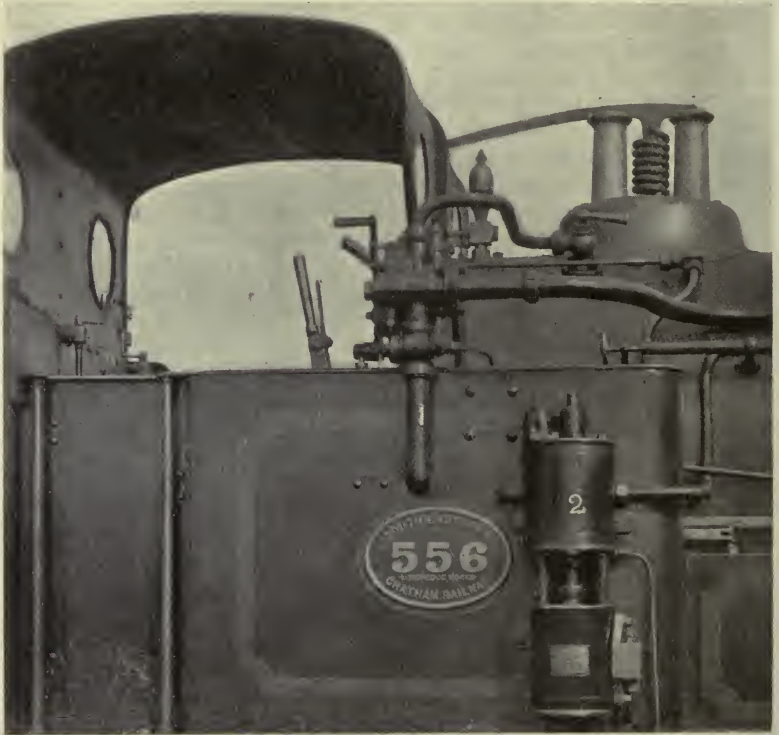
1. VACUUM BRAKE EJECTOR. 2. WESTINGHOUSE PUMP
