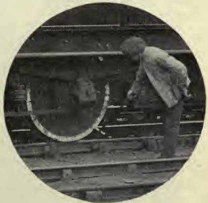
TRAIN EXAMINER—TESTING WHEELS (London, Tilbury, and Southend Railway)
