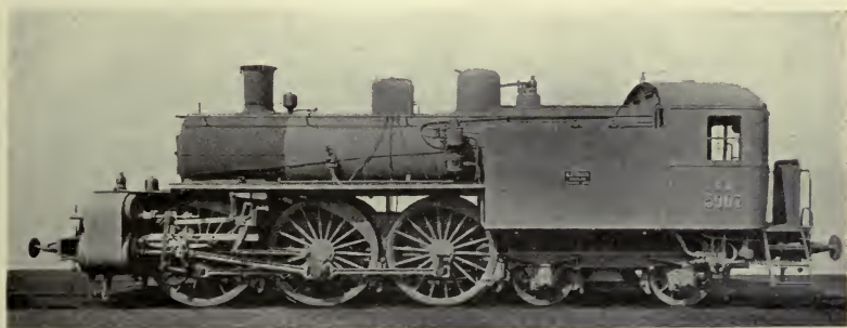
A BOLD DEPARTURE IN LOCOMOTIVE CONSTRUCTION. 4-6-0 FOUR-CYLINDER COMPOUND ENGINE (Italian Southern Railway)
