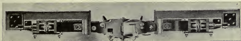
LAYCOCK'S COMBINATION VERTICAL-PLANE AUTOMATIC CENTRE COUPLER
