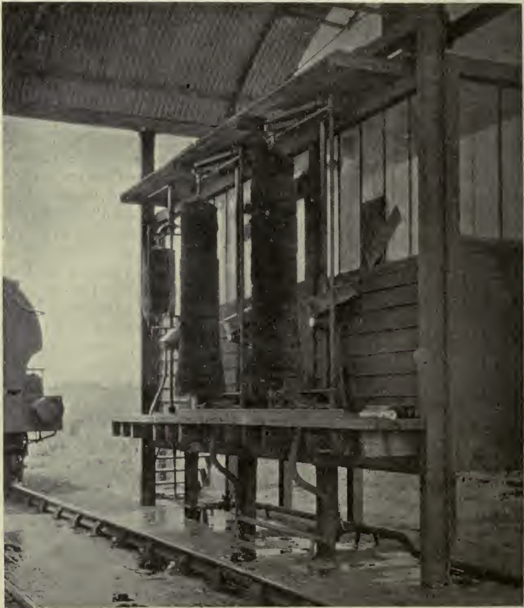
CARRIAGE CLEANING APPARATUS—REVOLVING BRUSHES (Great Western Railway)
