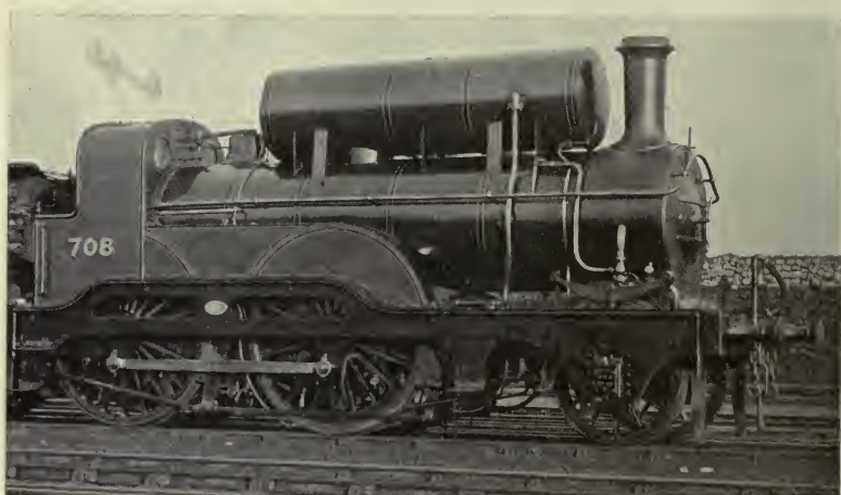
NO. 708, FITTED WITH THERMAL STORAGE TANK (Great Northern Railway)
