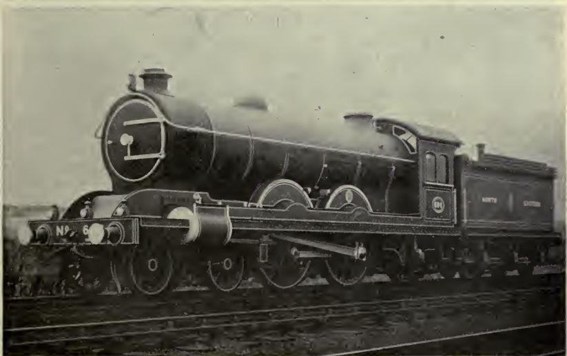
1. A "JENNY LIND." 2. POWERFUL MINERAL ENGINE, 0-8-0 3. PASSENGER EXPRESS LOCOMOTIVE, NO. 696, "ATLANTIC" TYPE (North Eastern Railway)
