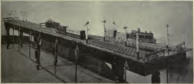
SIGNALLING INSTRUCTION MODEL (London and North Western Railway)
