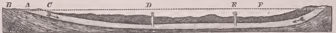
FIG. 1.—Ideal section illustrating the chief requisite conditions of artesian wells. A, a porous stratum; B and C, impervious beds below and above A, acting as confining strata; F, the height of the water-level in the porous bed A, or, in other words, the height of the reservoir or fountain-head; D and E, flowing wells springing from the porous water-filled bed, A. (According to T. C. Chamberlin.)
