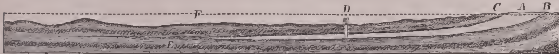
FIG. 2.—Section illustrating the thinning out of a porous water-bearing bed, A, inclosed between impermeable beds, B and C, thus furnishing the necessary conditions for an artesian fountain, D. (According to T. C. Chamberlin.)
