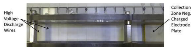
Fig. 3. ESP radionuclide collector under development for this work. ESP can achieve very high collection efficiencies (> 99.5%) across a wide range (30 nm to > 100 \mu\text{m} ) of particle sizes.
