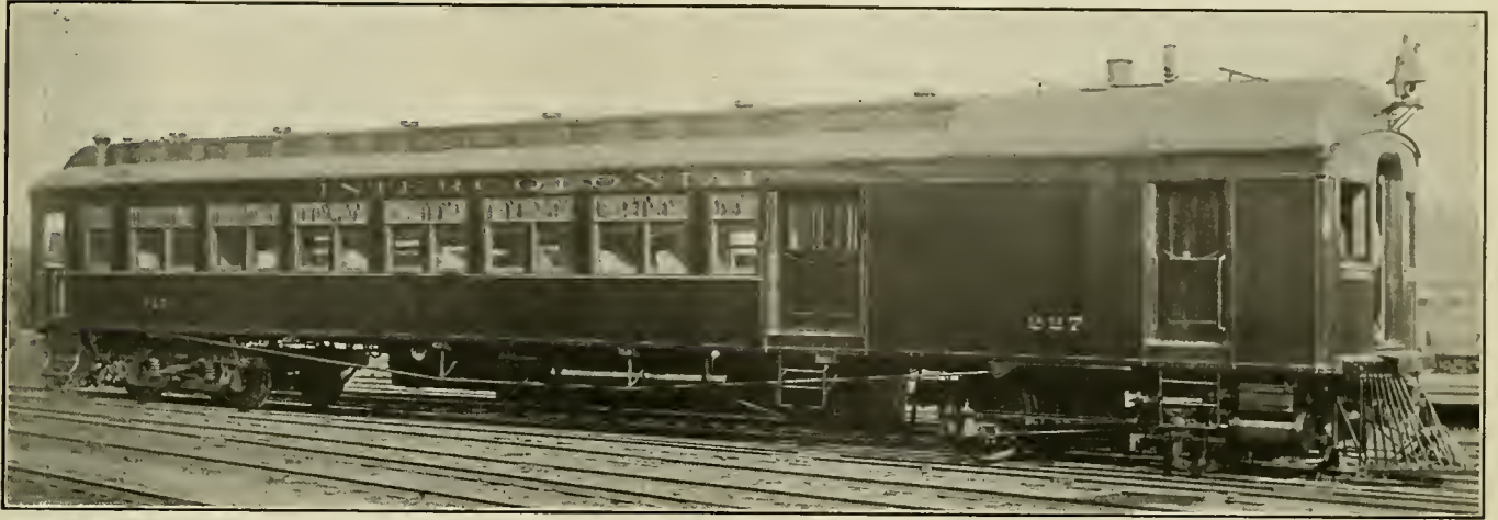
STEAM MOTOR CAR, INTERCOLONIAL RAILWAY.
