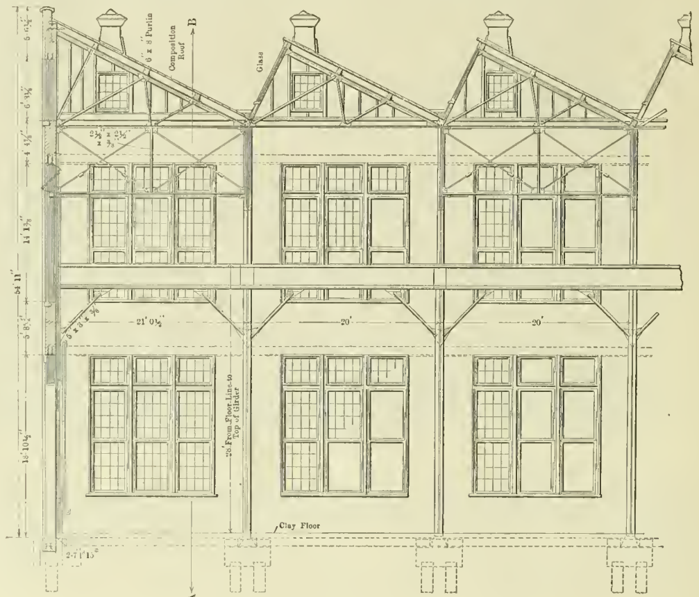
PART LONGITUDINAL SECTION OF FOUNDRY BUILDING.
