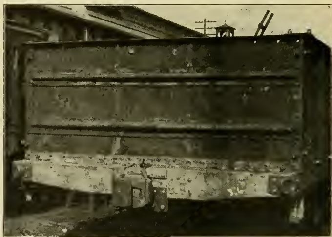
FIG. 24.—THE ENDS OF THE EARLIER GONDOLA CARS ARE BEING REINFORCED WITH HEAVY HORIZONTAL BRACES.
