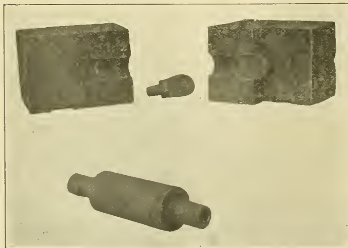
FIG. 2. DIES AND HEADER FOR FORGING SLING STAY I-BOLT.
