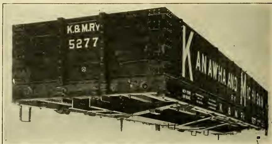
RALSTON STEEL UNDERFRAME AS A REPAIR FEATURE.
