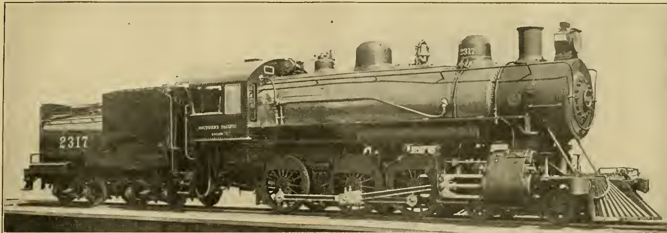
POWERFUL TEN-WHEEL OIL BURNING LOCOMOTIVE—SOUTHERN PACIFIC COMPANY.
