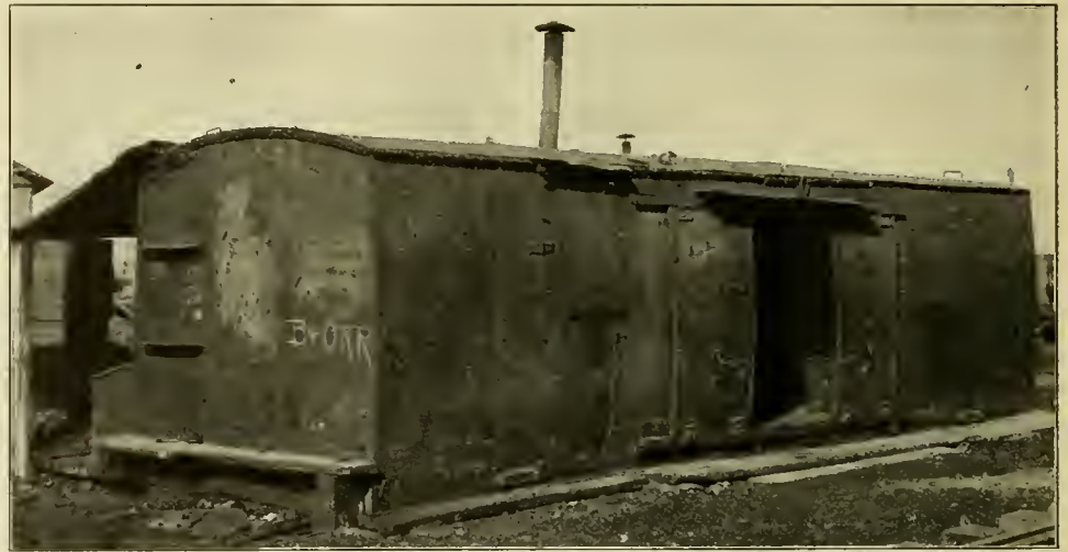
FIG. 7.—BODY OF ONE OF A SERIES OF IRON BOX CARS INTRODUCED ON THE BALTIMORE AND OHIO RAILROAD IN 1862.
