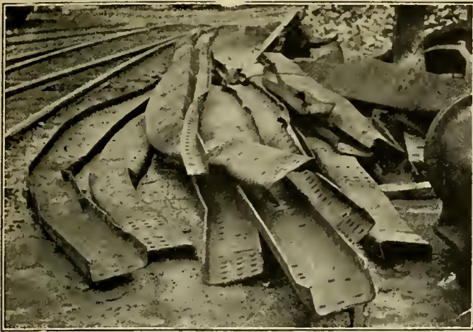
FIG. 30.—DAMAGED SIDE AND CENTER SILLS.
