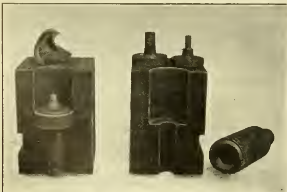
FIG. 4. DIES AND HEADER FOR VACUUM RELIEF VALVE.
