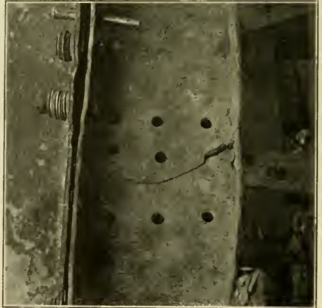
FIG. 44.—TORN BODY BOLSTER DIAPHRAGM.
