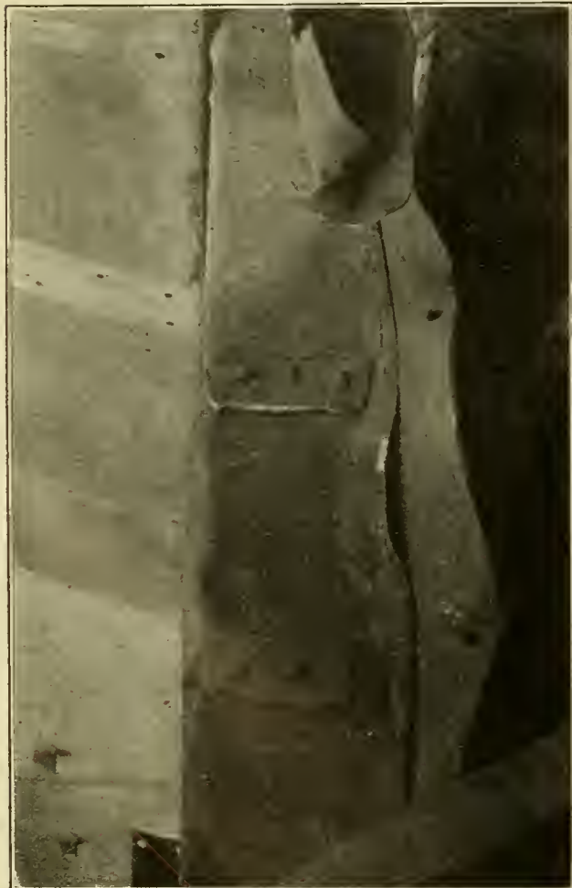
FIG. 46.—DRAFT SILLS TORN FROM THE BODY BOLSTER ON O-12 CONDOLA CAR.
