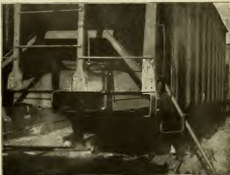
FIG. 26.—THE SILLS SHOWN IN FIG. 25 AFTER THEY WERE STRAIGHTENED.
