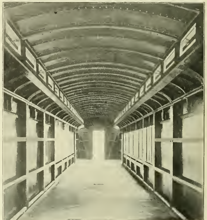
SIDE AND ROOF FRAMING—PENNSYLVANIA STEEL POSTAL CAR.
