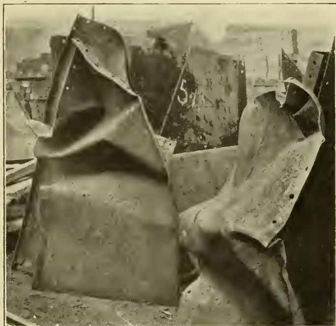
FIG. 27.—DAMAGED SIDE SHEETS.
