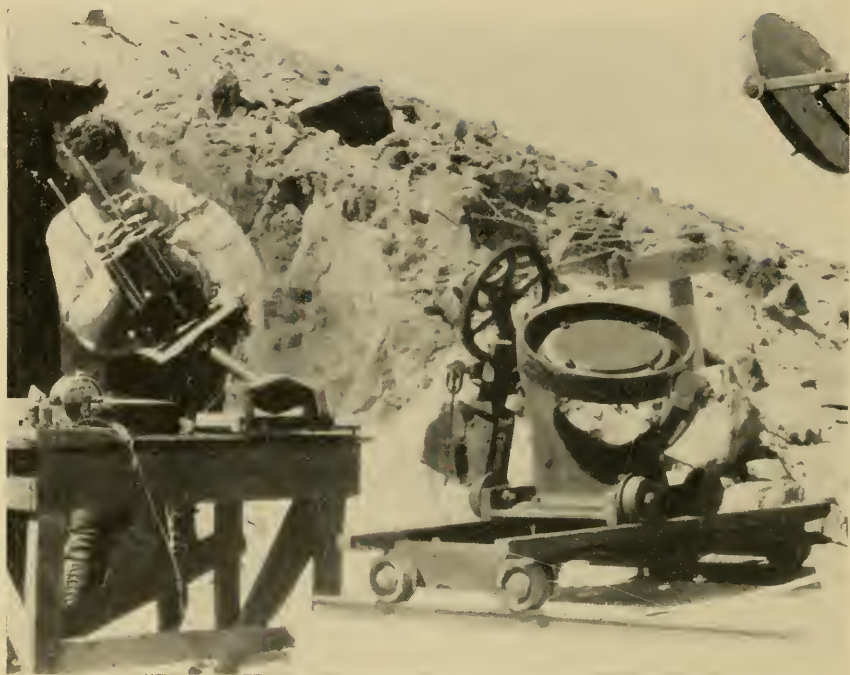
THE COELOSTAT AND THE PYRHELIOMETER JUST OUTSIDE THE TUNNEL AT MONTEZUMA, CHILE.
