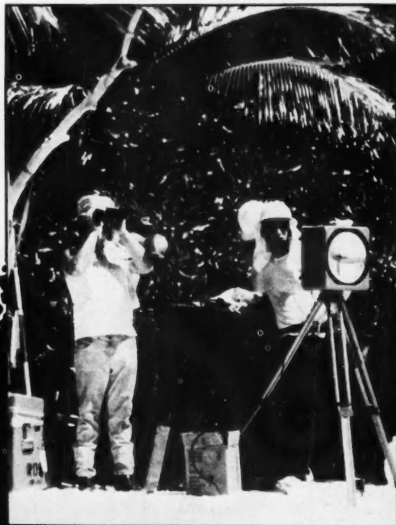
Surveyors use an electrotape to measure the distance across a Diego Garcia lagoon.
