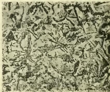
Glazed Northampton iron (Sample 3). Etched with 5 per cent. solution of nitric acid. Vertical illumination, magnified 75 diameters. Reduced by about one third in reproduction.
