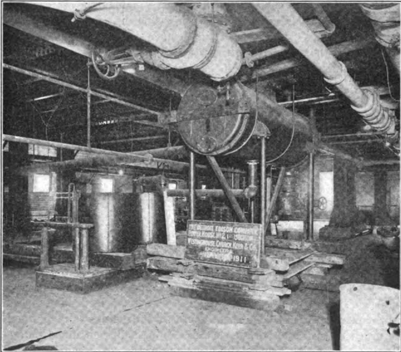
FIG. 10 SPECIAL CONDENSER AND WEIGHING APPARATUS FOR DETERMINING QUANTITY OF STEAM USED BY STOKER AUXILIARIES
