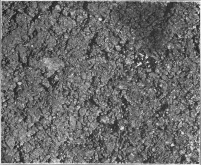
FIG. 13 PITCH-BOUND CORE WITH BONDED MOLDING SAND BASE INTENDED FOR HEAVY WORK
