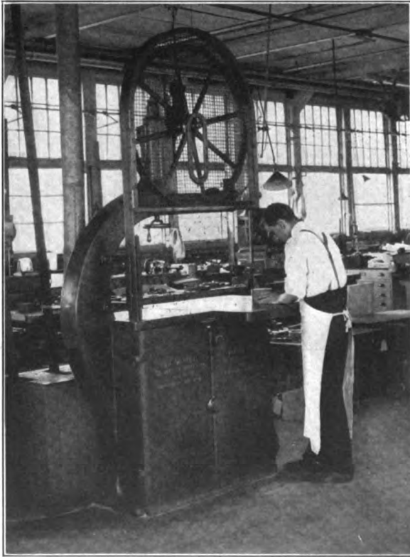
FIG. 61 BAND SAW COMPLETELY GUARDED
