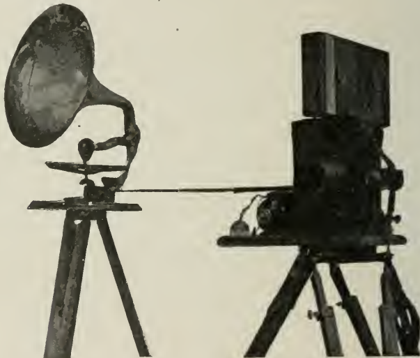
Fig. 112. The Recording Motion-Picture Camera Coupled to the Reproducing Graphophone for Producing the Picture Record of a Talking Picture
