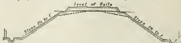
FIG. 11.—Type section of an embankment.
