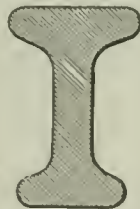
FIG. 8.—The bull-headed rail (62 lb per yard).
