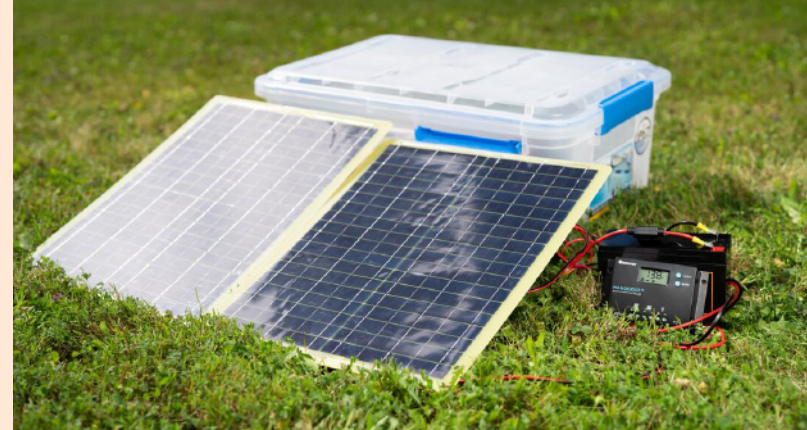
Example of the final system with panels tilted at 26 degrees to optimize their performance in Arcata, CA during summer months.
