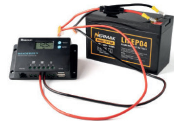
Charge controller connected to battery (through the fuse on the positive wire).
