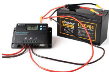
Charge controller connected to battery and now the solar panels.
