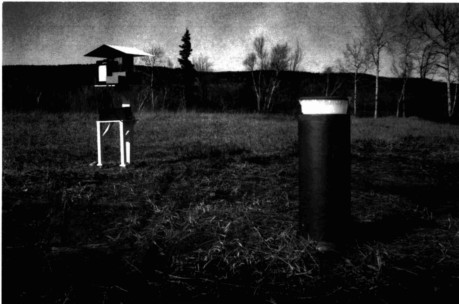
Fig. 4: Fallout collector and \Upsilon radiation monitor.
