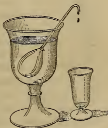
Osmose producing a continuous flow.
