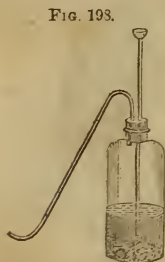
FIG. 193. Jar for making Carbonic Acid.
