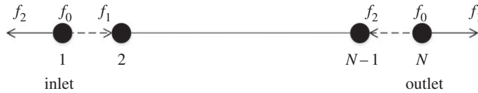
Figure 3. Distribution function at the inlet and outlet boundaries.
