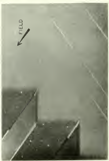
The domain structure of plate 4 was disturbed by applying small magnetic fields along two of the easy directions. Here we can see the way in which the domain walls move so that favored domains grow.
