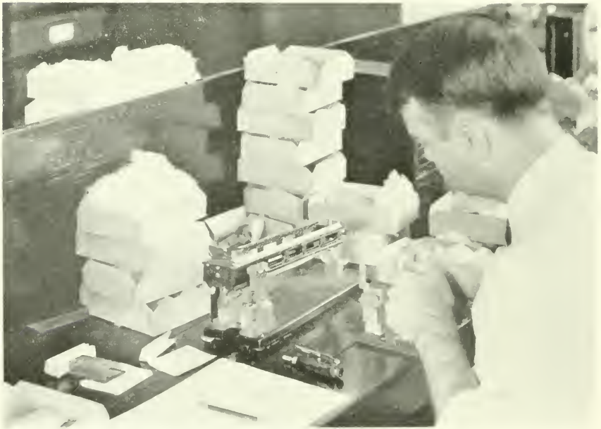
2. Technician determining the average fiber strength of prepared test specimens of cotton lint using the Pressley flat-unwrapped-bundle tester. The gauge spacing generally used between the two gripping jaws of the fiber bundle is either 0 or 1/8-inch. The strength results may be expressed as the initial Pressley index observed, or some other calculated index, or 1,000 pounds per square inch, or the new textile measure of grams per tex.
