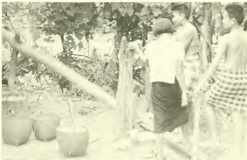
2. A foot-operated pestle drops on the rice in the container to the right and thus pounds off the hulls. Northeast Thailand.
