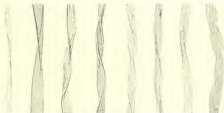
2. Composite photomicrograph of longitudinal views of fibers showing variations in degree of maturity or cell-wall thickening over a wide range as found in American upland cotton. Magnification in all cases X 165.
