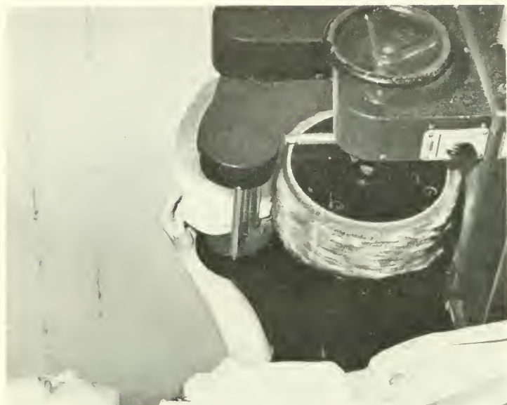
2. Technician blending a sample of ginned lint using the Gaus-Larrison mechanical cotton fiber blender. Owing to the great variations existing in the distribution and proportions of cotton fiber types throughout a sample, the determination of most fiber properties requires a preblending of the cotton in order to give representative and reliable test specimens.
