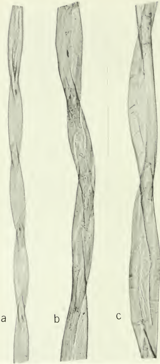
Composite photomicrograph of longitudinal views of mature cotton fibers of different botanical growths selected to represent a range in fineness: Specimen a is a fine fiber from Sea Island cotton Gossypium barbadense , staple length 1\frac{3}{4} inches; c is a very coarse fiber of the variety Garo Hill from Asian cotton G. herbaceum , staple length about \frac{5}{8} inch; and b is a fiber of intermediate fineness between a and c from American upland cotton G. hirsutum , staple length 1\frac{3}{8} inches. Magnification in all cases X 475.
