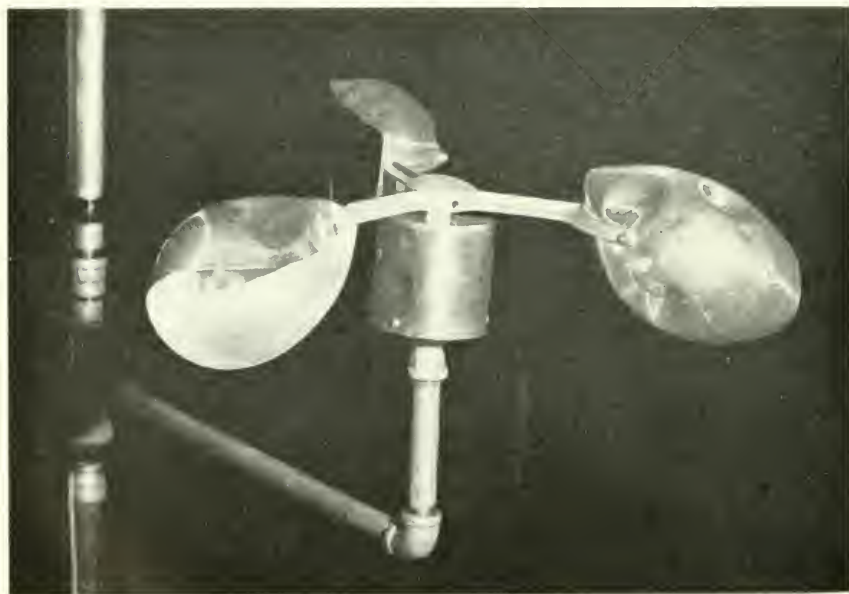
2. Hail damage to 3-cup anemometer located at Grand Island Airport, June 27, 1959. (Frontier Airlines photograph.)
