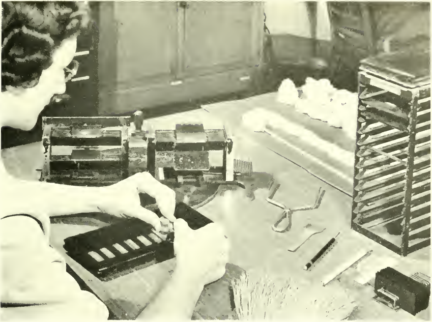
1. Technician performing fiber-length tests on prepared test specimens of cotton lint using the Suter-Webb Duplex Cotton Fiber Sorter. This instrument permits a stratification of the many fiber-length groups occurring in any sample of cotton and the formation of a cotton-fiber-length array from which the length distribution can be accurately evaluated for the entire sample, and various statistical values calculated for its central tendencies and variability.
