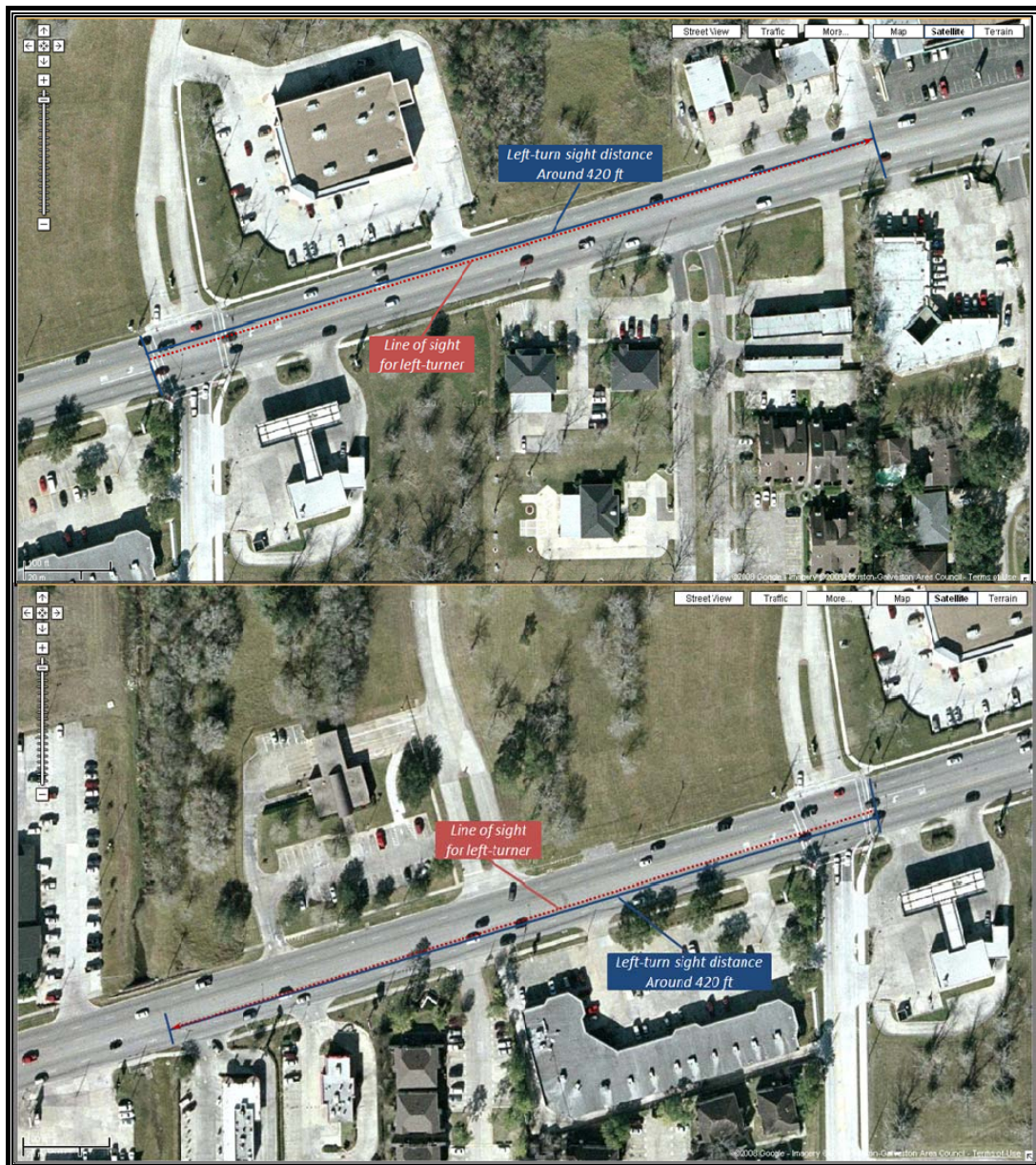
Figure 83: Sight Distances for the Left-Turn Movements at WB and EB Approaches of the Intersection at FM 518 and Calder Drive
