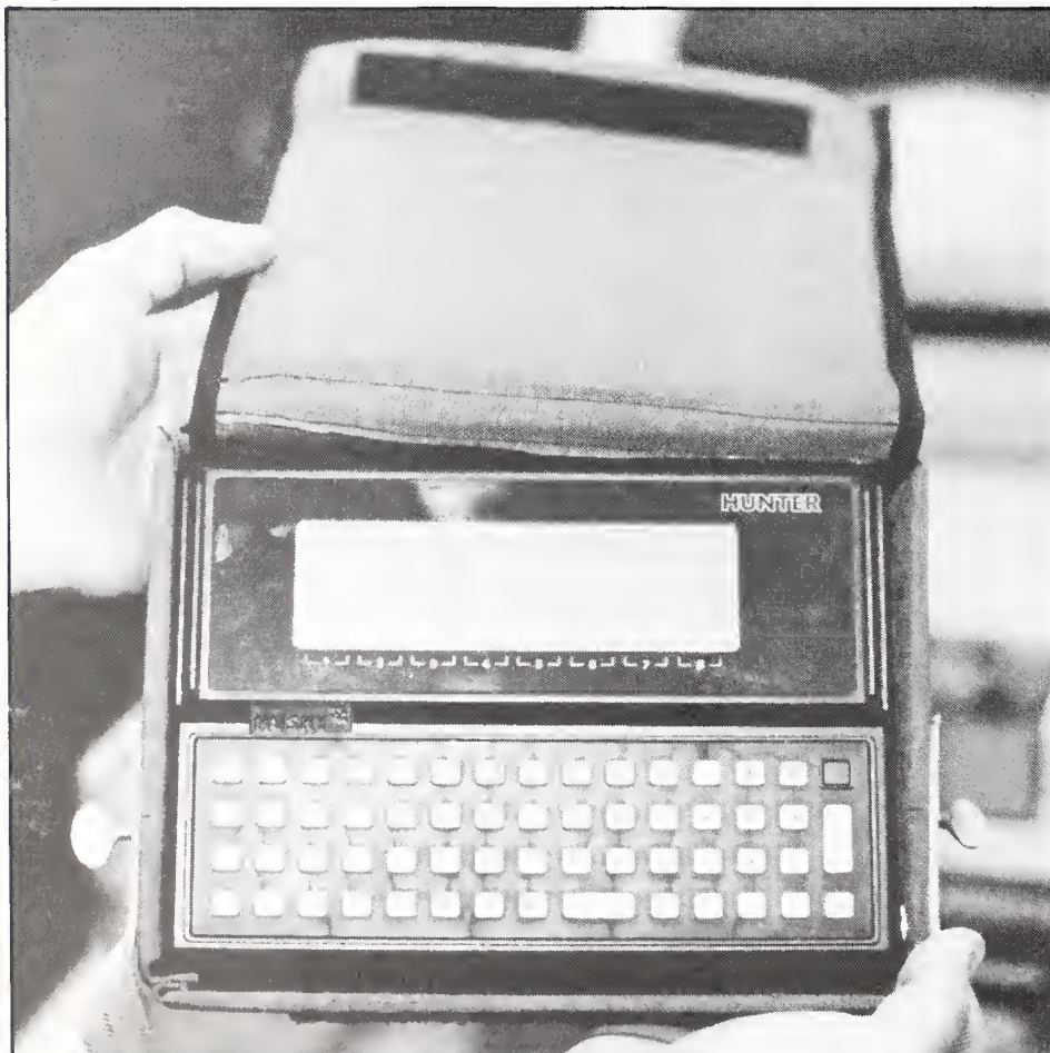
The Husky Hunter in a cloth carrying case designed for field use.
