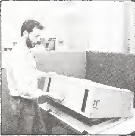
The travel case serves as a portable work station, about 2 feet wide and 2 feet deep. It fits on top of most motel furniture and in the back of a vehicle similar to a Blazer or Jeep. When loaded, it weighs less than 40 pounds.
