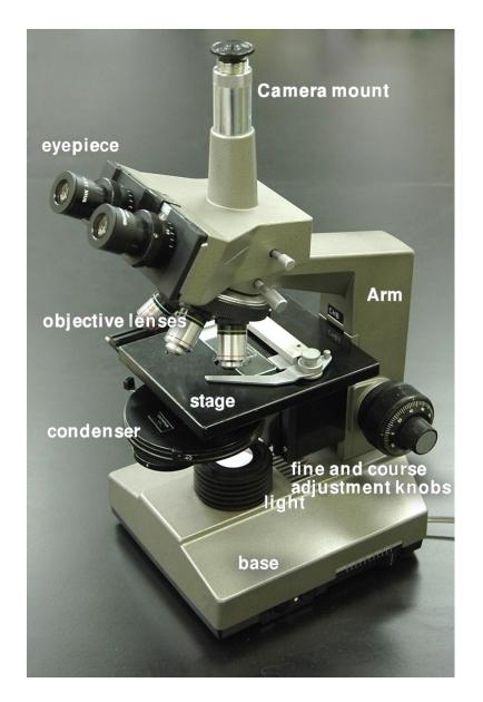
Figure 1.30: Compound light microscopes use lenses to focus light. Typical magnification of a light microscope is up to 1500x. This microscope has two optical lenses and is called a stereo microscope. The various parts of the microscope are labeled. (41)
