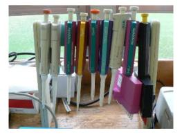
Figure 1.29: Pipettes are small, but important tools in many biology labs. Micropipettes, such as these here, are calibrated to measure very small amounts of liquids. For example, 100 microliters (100  $\mu$ L) which is about half the volume of your little finger tip; or even 1  $\mu$ L, which is smaller than a drop of water. (16)
