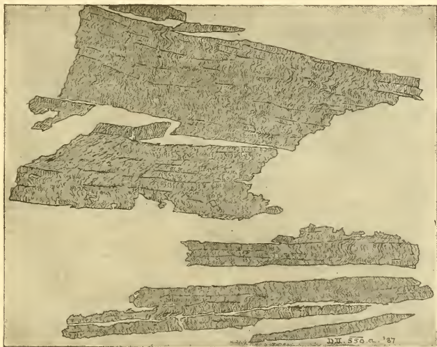
FIG. 53.—Thin section of sericite-chlorite-schist from locality 550, about one-quarter mile south of Greylock summit, enlarged 2\frac{1}{2} diameters, showing a coarse slip cleavage crossing a very minutely plicated stratification. In preparing the slide fractures occurred mainly in the direction of the cleavage, here the direction of least resistance. From a photograph.
