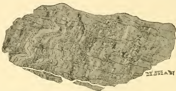
FIG. 73.—Thin section of albitic sericite-schist from locality 542, between Greylock summit and Saddle Ball, enlarged \frac{1}{4} diameters. A typical specimen of the Greylock schist, showing the minute plications, the quartz lamina, the slip cleavage with the albite interspersed. (From a photograph.)
