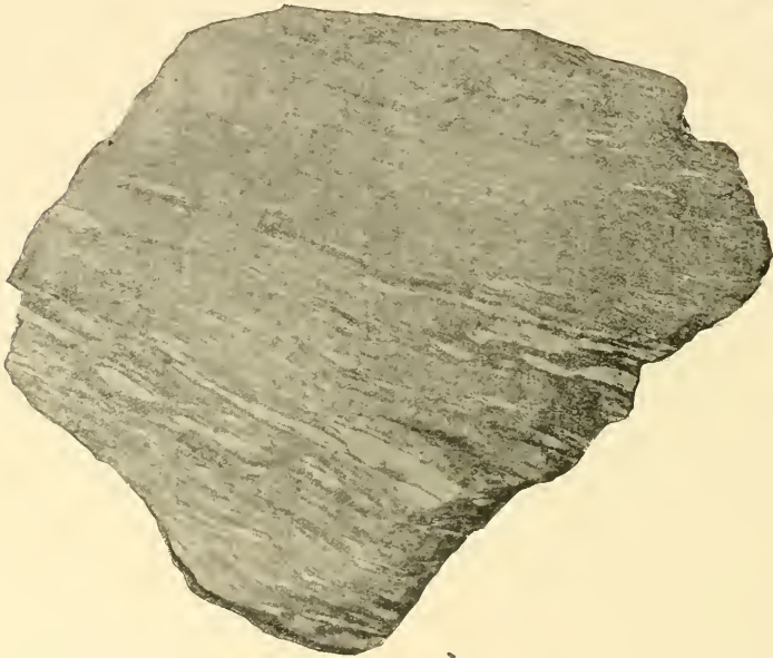
FIG. 23.—Albite schist (Hoosac schist). Dump, Central shaft. About one-eighth natural size. Here the quartz lenses are again prominent. It is found that they are always parallel to the stratification.
