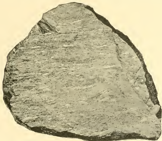
FIG. 21.—Albite schist (Hoosac schist). Dump, Central shaft. One twelfth natural size. This is the type with thin flat quartz layers (the white streaks) and gentle crumpling.
