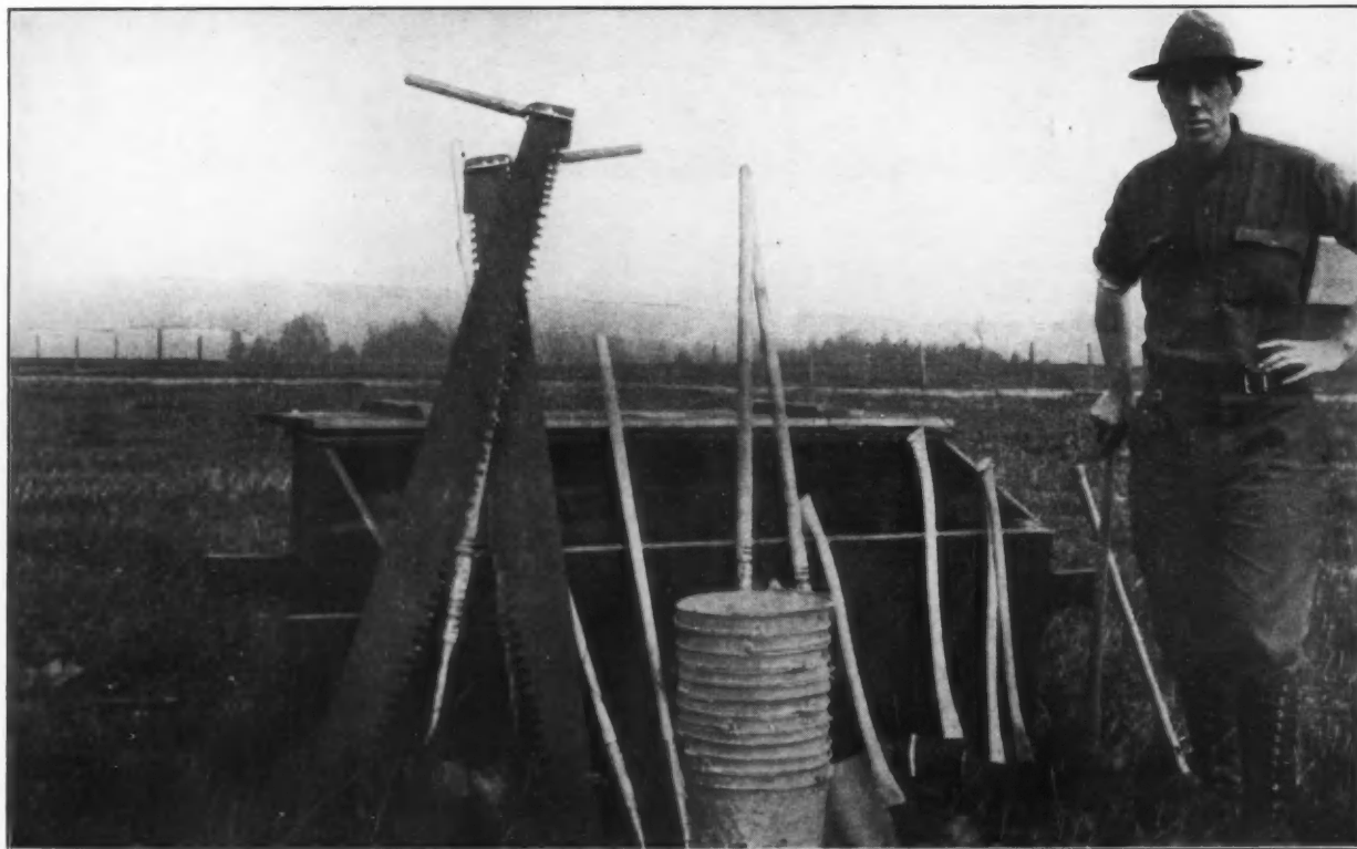
TYPE OF FIRE TOOL BOX KEPT IN TOWERS, CAMPS, STORE HOUSE, OR PLACED ALONG ROADS WHERE FIRE THREATENS. IMPLEMENTS FOR 20 MEN. AUTHOR AT RIGHT.
